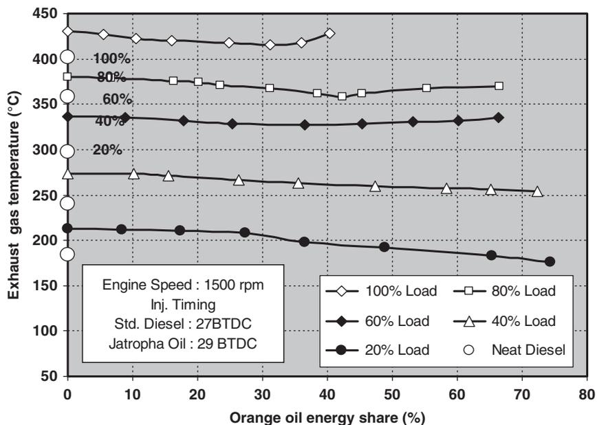
Fig. 4 Variation of exhaust gas temperature with orange oil energy share
