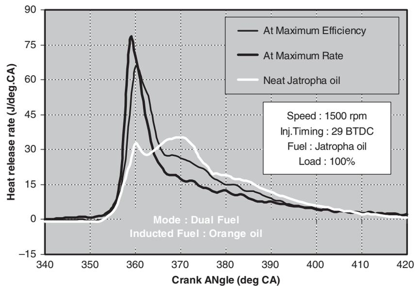
Fig. 14 Variation of heat release rate with JO in dual-fuel operation at 100 per cent load
