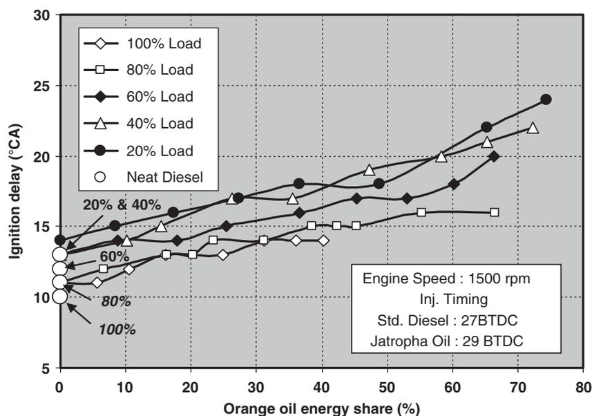
Fig. 9 Variation of ignition delay with orange oil energy share
