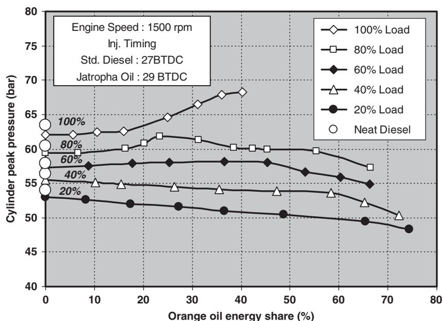
Fig. 10 Variation of cylinder peak pressure with orange oil energy share
