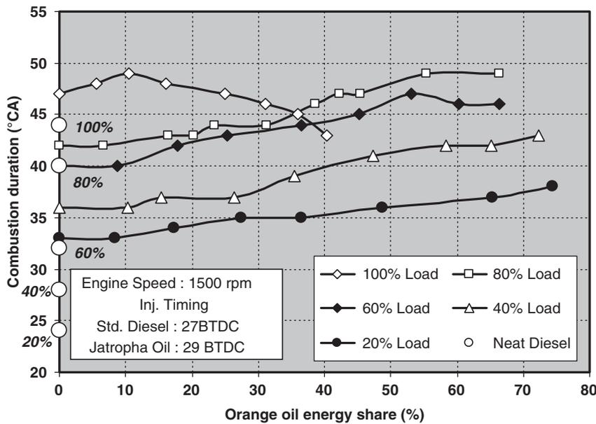
Fig. 12 Variation of combustion duration with orange oil energy share
