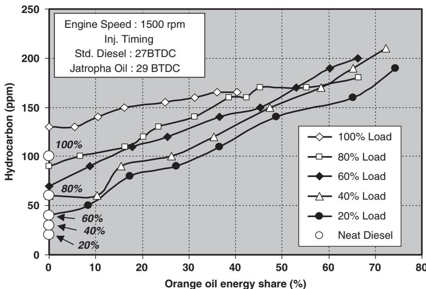
Fig. 6 Variation of hydrocarbon emissions with orange oil energy share
