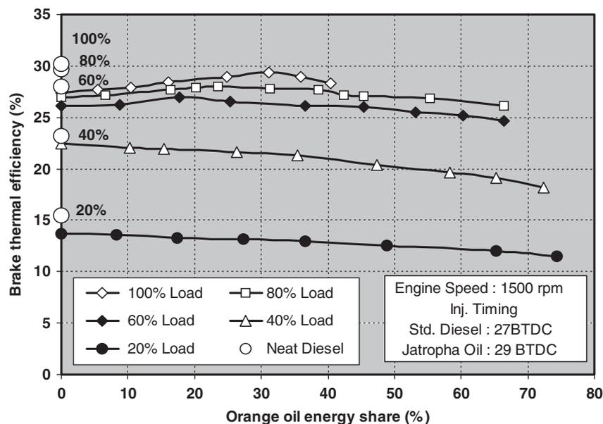
Fig. 2 Variation of brake thermal efficiency with orange oil energy share
