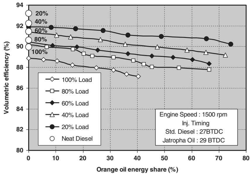
Fig. 3 Variation of volumetric efficiency with orange oil energy share
