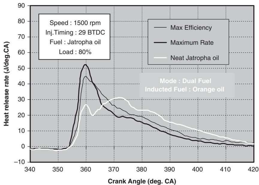
Fig. 15 Variation of heat release rate with JO in dual-fuel operation at 80 per cent load
