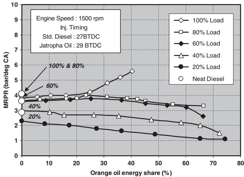
Fig. 11 Variation of maximum rate of pressure rise with orange oil energy share
