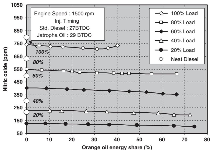
Fig. 8 Variation of nitric oxide with orange oil energy share
