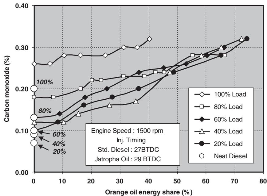
Fig. 7 Variation of carbon monoxide with orange oil energy share
