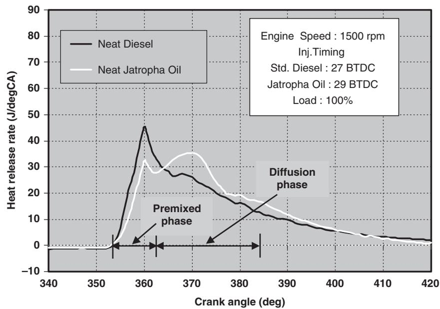
Fig. 13 Variation of heat release rate with neat diesel and neat JO at 100 per cent load
