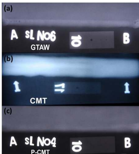
Fig. 1 – X-ray radiograph of P91 steel joint produced by (a) GTAW, (b) CMT and (c) P-CMT processes.
