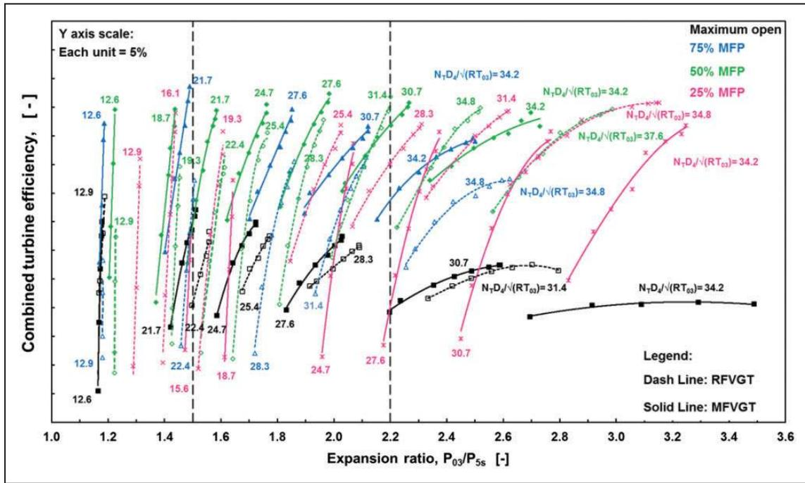
**Figure 10.** Combined turbine efficiency vs. expansion ratio for RFVGT and MFVGT at different opening positions of nozzle vanes: similar MFP openings. MFVGT: mixed flow variable geometry turbine; RFVGT: radial flow variable geometry turbine; MFP: mass flow parameter.
