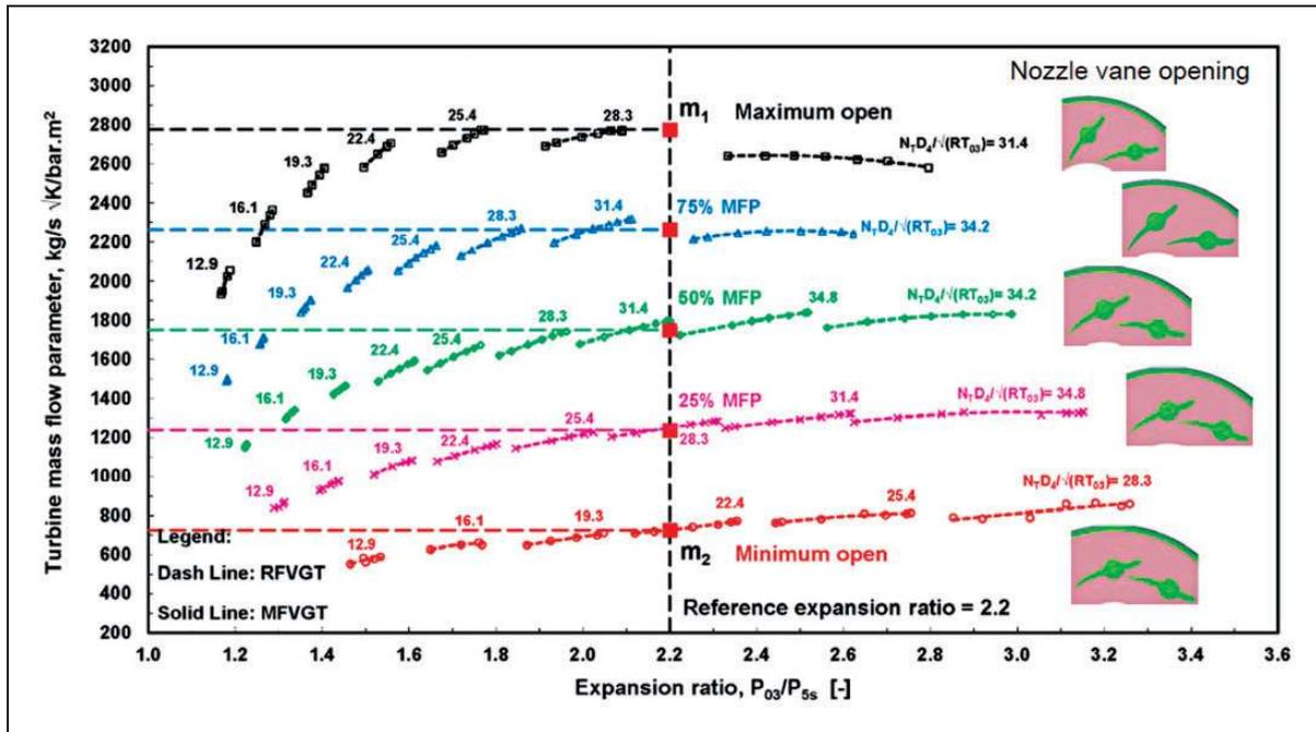
**Figure 6.** Performance of RFVGT at different opening positions of nozzle vanes.
