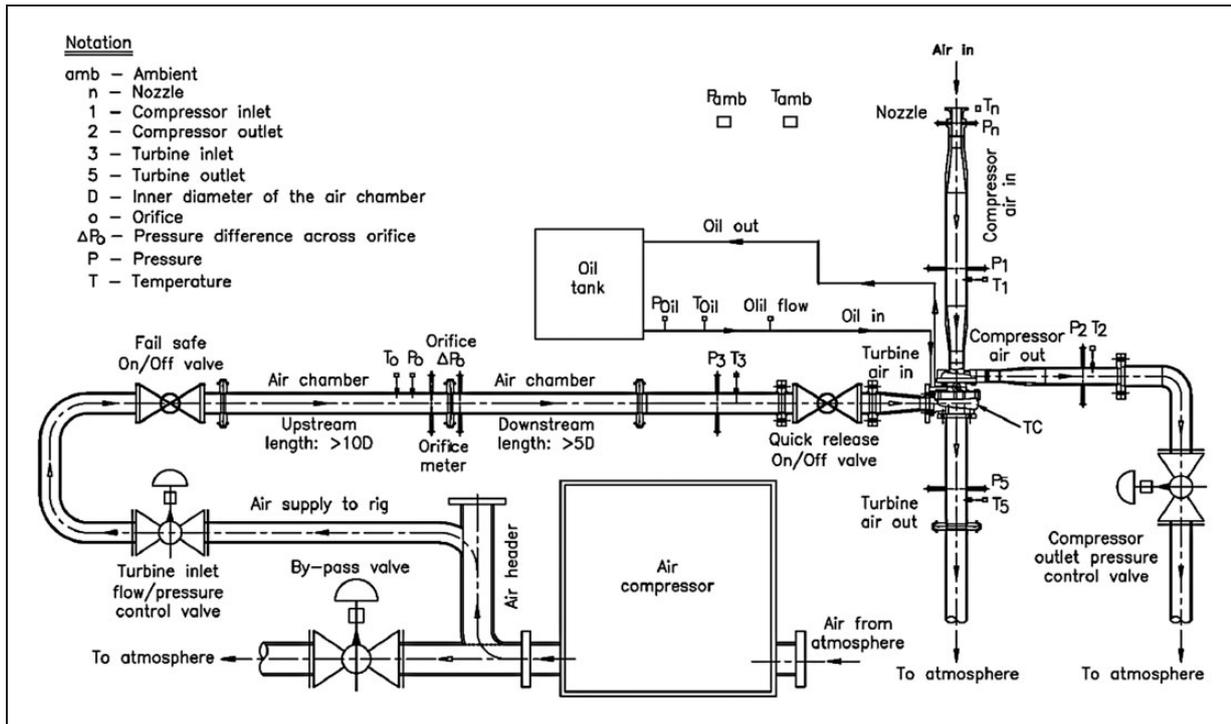
Figure 5. Turbocharger cold air test rig layout.
