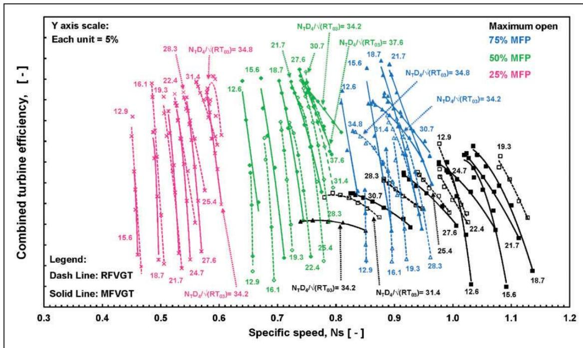
**Figure 13.** Combined turbine efficiency vs. turbine specific speed for RFVGT and MFVGT at different opening positions of nozzle vanes: similar MFP openings.
