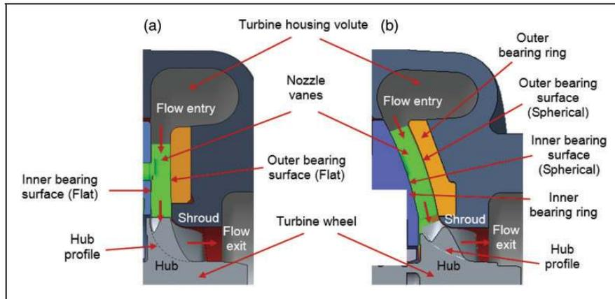
**Figure 2.** Turbine stage for RFVGT and MFVGT: (a) radial flow VGT; and (b) mixed flow VGT.
