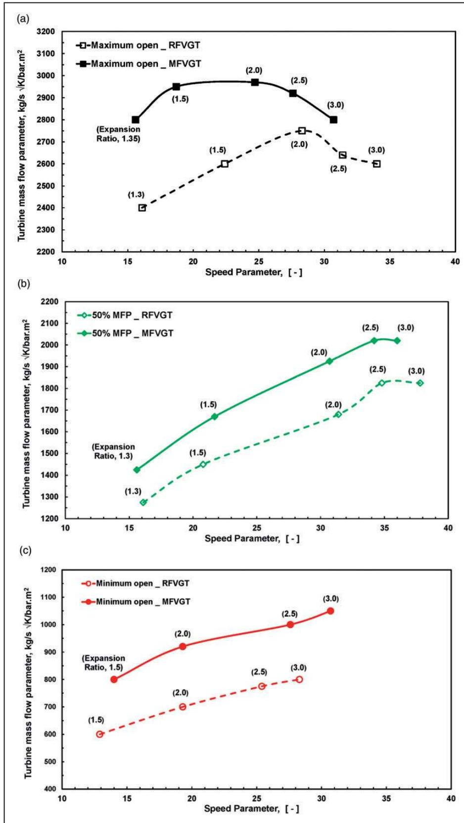
**Figure 8.** Turbine mass flow parameter vs. turbine speed parameter for RFVGT and MFVGT at different opening positions of nozzle vanes: (a) maximum nozzle vanes open; (b) 50% MFP nozzle vane open; and (c) minimum nozzle vane open. MFVGT: mixed flow variable geometry turbine; RFVGT: radial flow variable geometry turbine; MFP: mass flow parameter.
