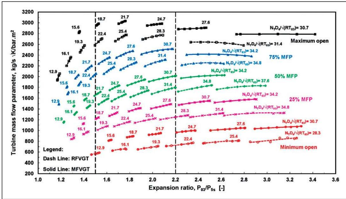
**Figure 7.** Turbine mass flow parameter vs. expansion ratio for RFVGT and MFVGT at different opening positions of nozzle vanes. MFVGT: mixed flow variable geometry turbine; RFVGT: radial flow variable geometry turbine.
