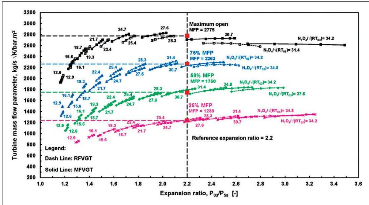
**Figure 9.** Turbine mass flow parameter vs. expansion ratio for RFVGT and MFVGT at different opening positions of nozzle vanes: similar MFP openings.
