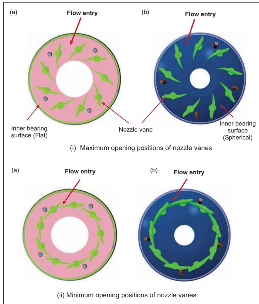
**Figure 4.** Side views of the (a) RFVGT and (b) MFVGT geometries at maximum and minimum opening positions of nozzle vanes.
