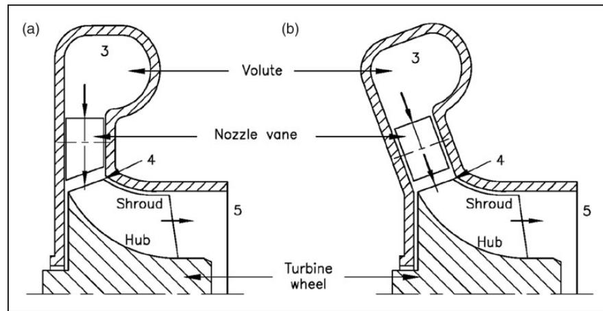
**Figure 1.** Possible options of nozzle vanes for a mixed flow turbine: (a) vane with flat hub/shroud surface; and (b) vane with inclined hub/shroud surface.
