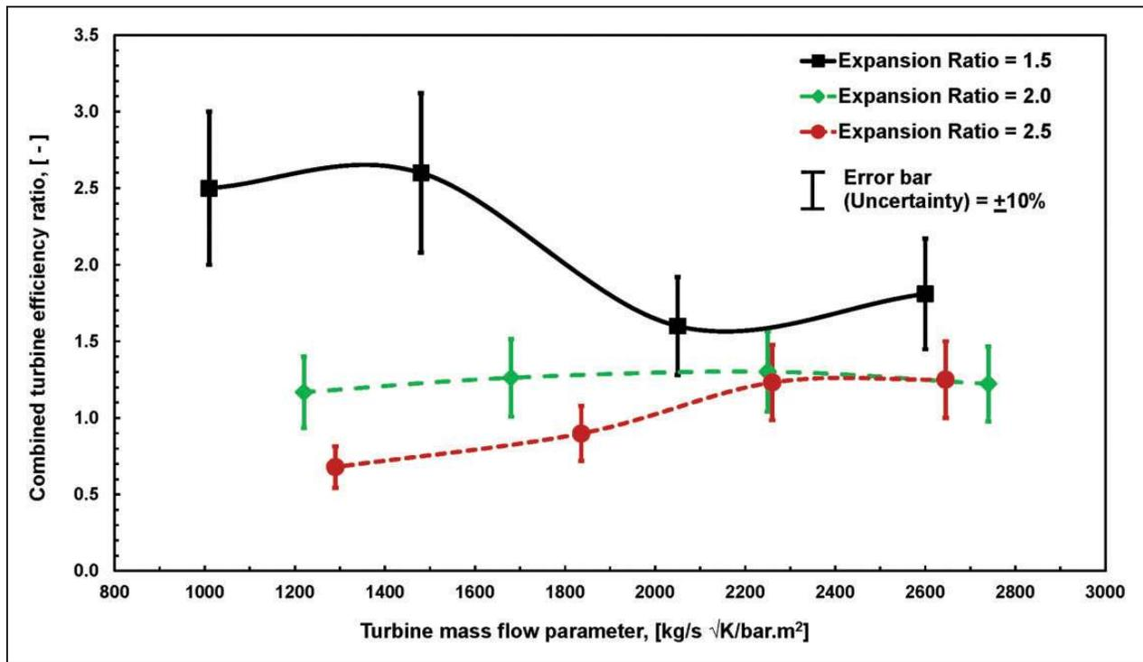
**Figure 11.** Ratio of combined turbine efficiency vs. turbine mass flow parameter at different expansion ratios for RFVGT and MFVGT (at different opening positions of nozzle vanes: for similar MFP openings).
