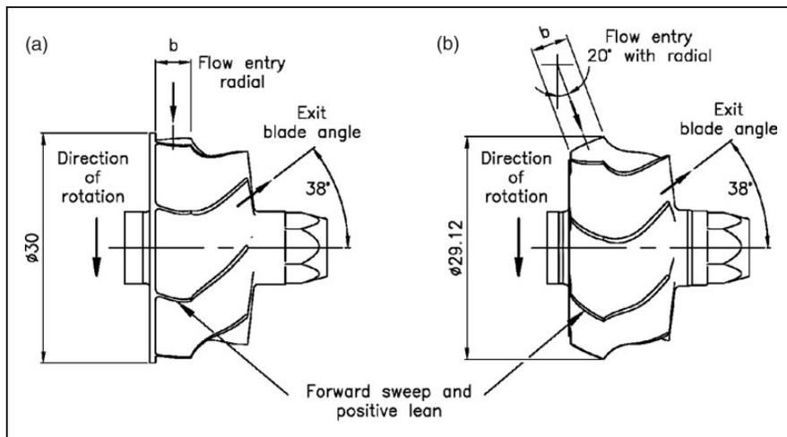
**Figure 3.** Schematic of the radial flow and mixed flow turbine wheel geometry: (a) radial flow turbine wheel; and (b) mixed flow turbine wheel.
