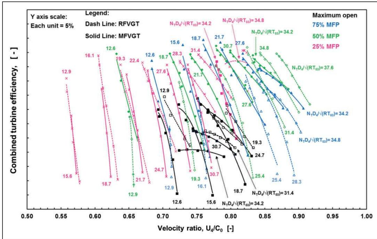
**Figure 12.** Combined turbine efficiency vs. velocity ratio for RFVGT and MFVGT at different opening positions of the nozzle vanes: similar MFP openings.
