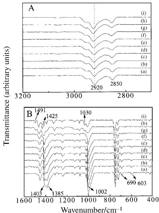
**Fig. 5** Variable temperature FTIR spectra for AgMBT in (A) the high wavenumber and (B) the low wavenumber region. The temperatures are: (a) 298, (b) 323, (c) 348, (d) 373, (e) 398, (f) 423, (g) 448, (h) 473 K and (i) cooling back to 298 K, respectively.
