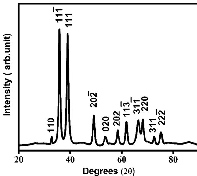
**Figure 1.** XRD pattern of CuO nucleated using higher concentration of precursors (30 mM Cu(OAc)<sub>2</sub>·2H<sub>2</sub>O and 180 mM NaOH) exhibiting monoclinic phase (Space group: C 2/c,#15).
