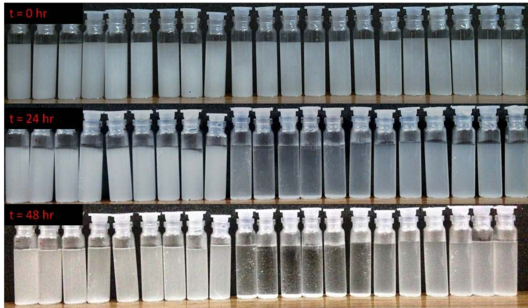
Figure S1. Heteroaggregation of aqueous dispersions of oppositely charged polystyrene latex particles of diameter 2.2\ \mu\text{m} (+) and 3.0\ \mu\text{m} (-), initially and one and two days later. From left to right, \phi_p = 0, 0.013, 0.020, 0.048, 0.063, 0.091, 0.167, 0.200, 0.250, 0.333, 0.500, 0.667, 0.750, 0.800, 0.833, 0.909, 0.938, 0.952, 0.980, 0.987 and 1.000 respectively. Total particle concentration is 0.1\ \text{w/v}\% ( \approx 6.7 \times 10^7 per mL of water phase), \text{pH} = 7 . Aggregation leading to significant sedimentation is observed at intermediate compositions 0.333 < \phi_p < 0.833 .
