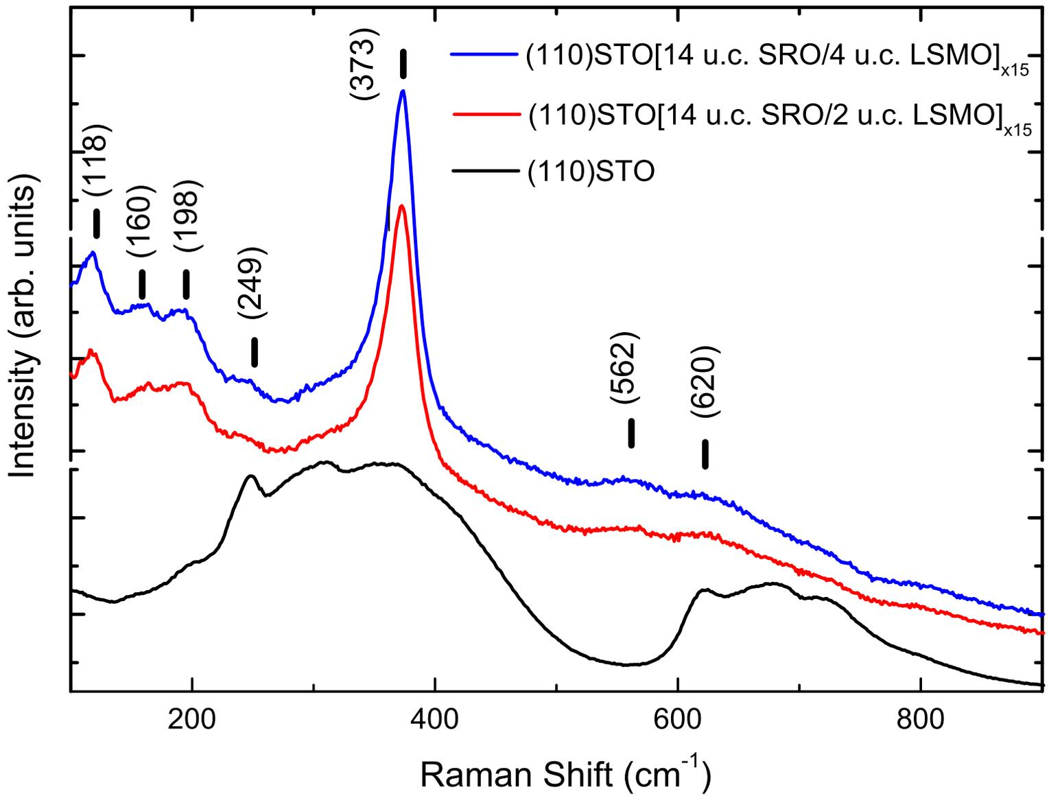
Figure 2: Raman spectra of (110) oriented STO substrate and superlattices with  $n = 2$  and 4.
