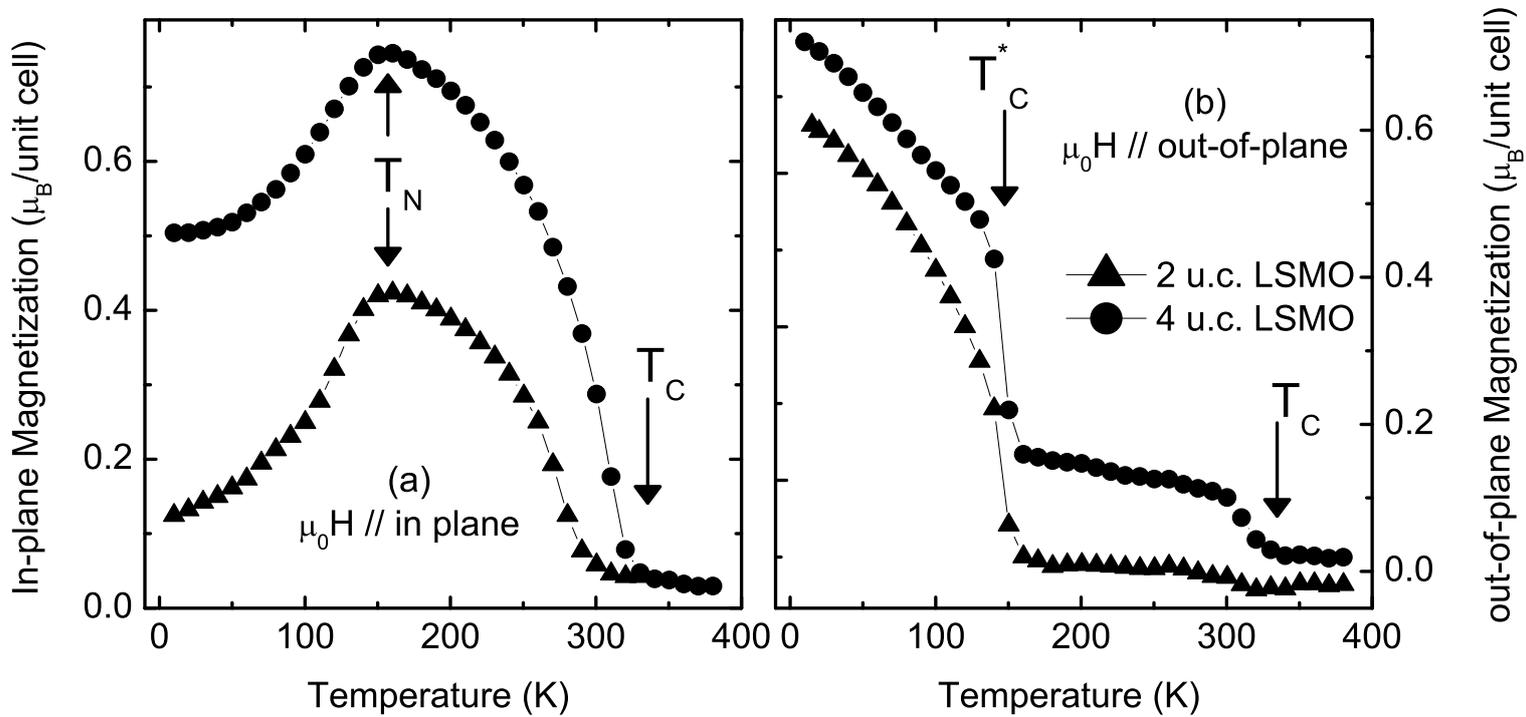
Figure 3: Temperature dependent 0.1 tesla field cooled (a) in-plane magnetization and (b) out-of-plane magnetization of the superlattices with  $n = 2$  and  $4$ . The arrows indicate the  $T_C$ ,  $T_C^*$ , and  $T_N$ .
