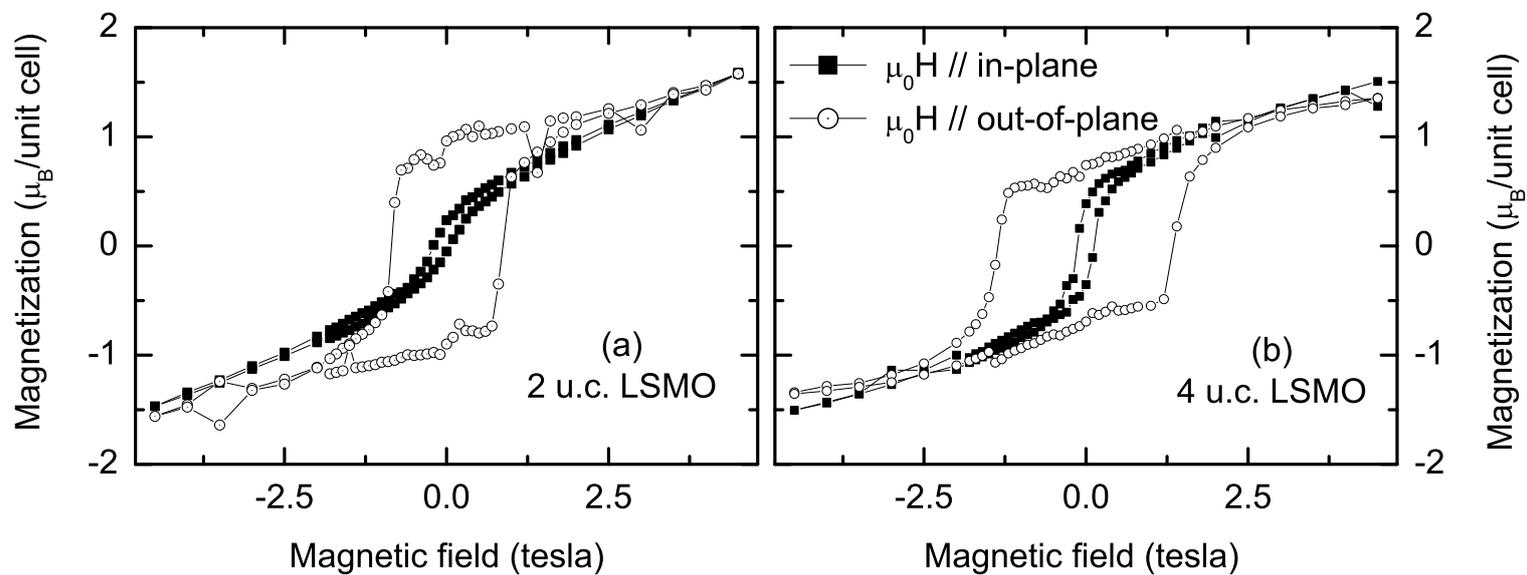
Figure 4: Field dependent magnetization at 10 K with field oriented along the plane and out-of-plane of (a) (110)STO/[14-u.c. SRO/2-u.c. LSMO]<sub>x15</sub> and (b) (110)STO/[14-u.c. SRO/4-u.c. LSMO]<sub>x15</sub> superlattices.
