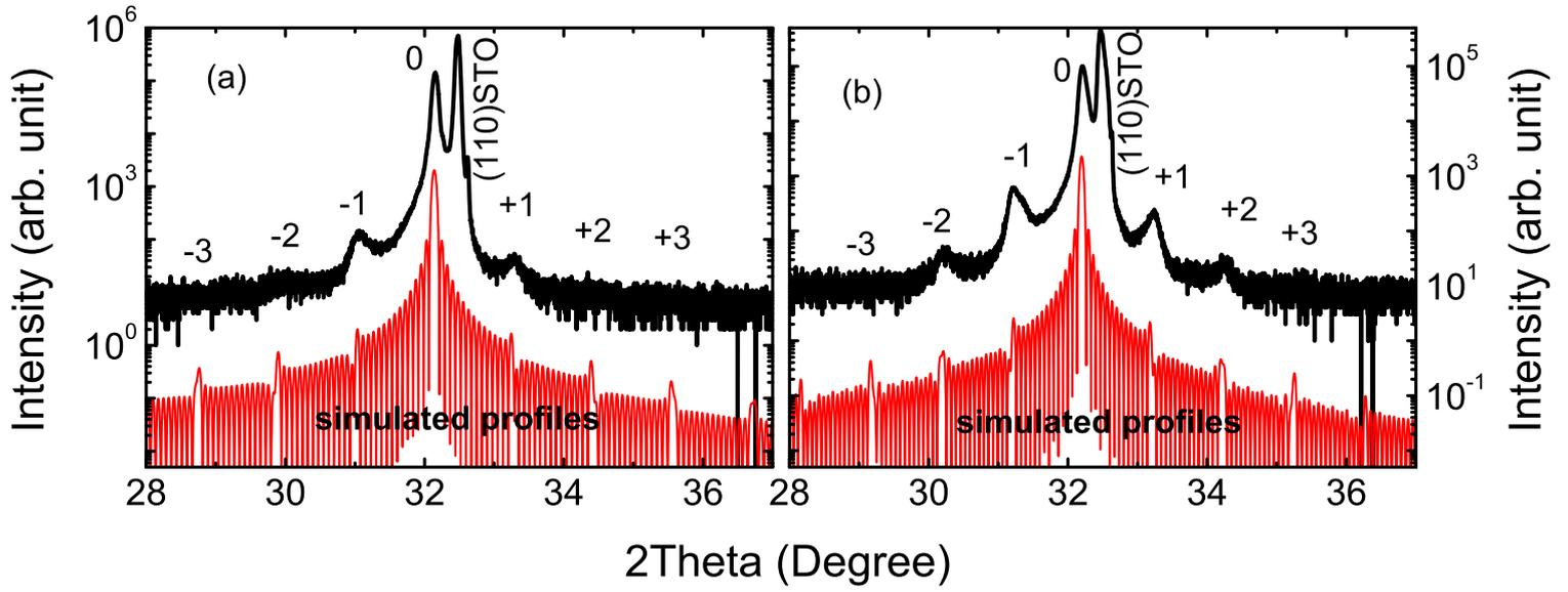
Figure 1: The  $\theta$ - $2\theta$  x-ray diffraction profiles and simulated spectra of (a) (110)STO/[14-u.c. SRO/2-u.c. LSMO] $_{x15}$  and (b) (110)STO/[14-u.c. SRO/4-u.c. LSMO] $_{x15}$  superlattices. The (110) Bragg's reflection of STO as well as the satellite peaks of the superlattice are indicated.
