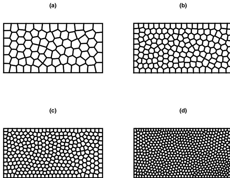
Figure 12: Sample meshes for the two dimensional cantilever beam problem containing: (a) 80, (b) 160, (c) 320 and (d) 640 polygons.
