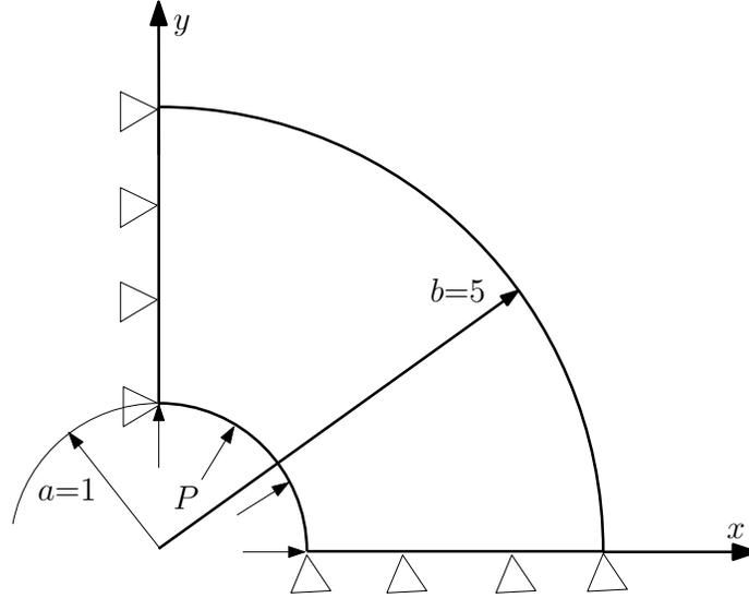
Figure 18: Thick-walled cylinder subjected to internal pressure.
