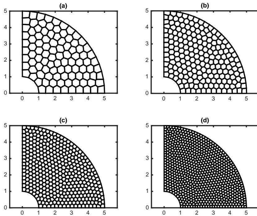
Figure 19: Representative meshes for the thick-walled cylinder containing:
