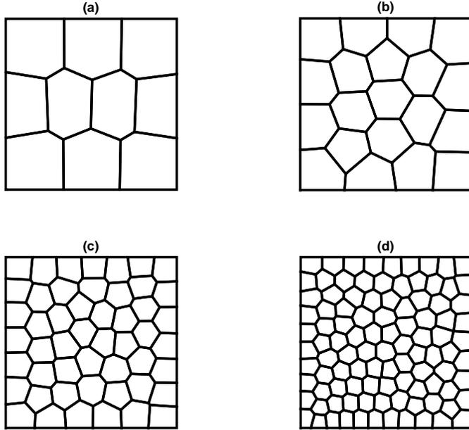
Figure 7: Square domain discretized with polygonal elements. Representative meshes containing (a) 10, (b) 20, (c) 50 and (d) 100 polygons.
