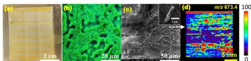
**Figure 3.** Comparative visualization of biofilms. (a) Photograph of RO membrane after biofilm growth (6 days). Marks on the membrane are due to the spacers used. (b) Dark field microscopic image of the biofilm (1 day growth). (c) SEM image of the biofilm (1 day growth). (d) Positive mode DESI MS image of the ion  $m/z$  673.4 (Rha-Rha-C10-C10 expressed on the biofilm after 1 day growth). DESI MS image is color coded, and the color code is shown on the right.
