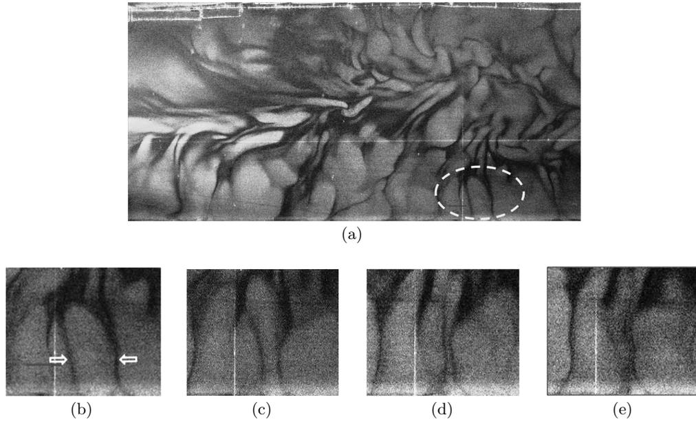
FIGURE 5. Dynamics of plumes in a low shear region at  $Pr = 0.74$  and  $Ra_w = 2.54 \times 10^8$ ; (a), The instantaneous planform in half the cell area of size  $985\text{mm} \times 477\text{mm}$ ; (b) to (e), merging sequence in a region of size  $162\text{mm} \times 135\text{mm}$  that has negligible shear, marked with a dashed ellipse in (a). The images (b) to (e) are separated by  $0.4\text{s}$ .
