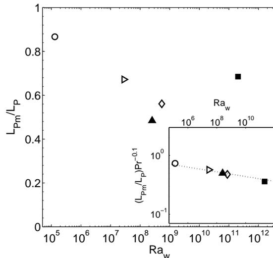
FIGURE 17. Variation of the ratio of the length of plumes that are merging in a planform to the total length of plumes in the planform ( $L_{pm}/L_p$ ) with  $Ra_w$ . The open symbols indicate thermal convection experiments in water for  $Pr = 3.6$  to  $5.3$  for the following layer heights; ○,  $H = 50$ mm; ▷,  $H = 100$ mm; ◊,  $H = 150$ mm; and ◊,  $H = 210$ mm. ▲,  $Pr = 0.73$ ; ■,  $Sc = 600$ . The inset shows the scaling of  $L_{pm}/L_p$  as per (5.6).
