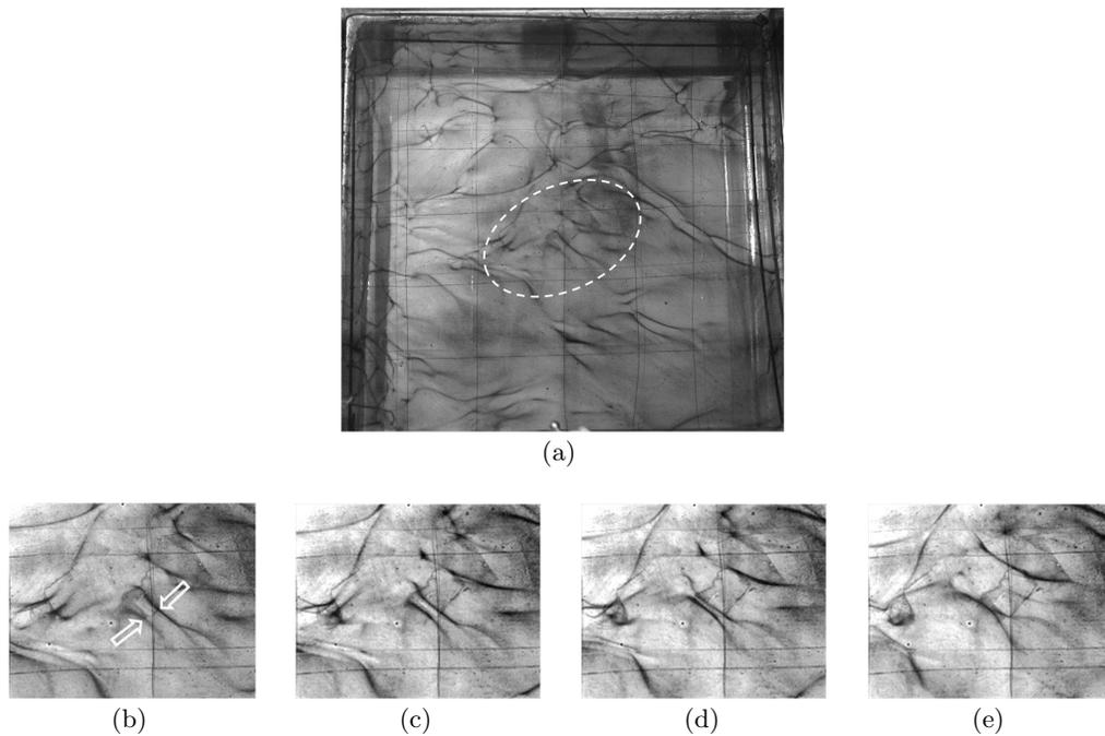
FIGURE 6. Dynamics of plumes in a low shear region at  $Pr = 4.7$ , and  $Ra_w = 2.65 \times 10^8$ ; (a), the instantaneous planform of the entire cell area of size  $298\text{mm} \times 287\text{mm}$ ; (b) - (e), merging sequence in the marked region in (a) with negligible shear; The images are of size  $100\text{mm} \times 77\text{mm}$  at times  $t = 0\text{s}, 1.5\text{s}, 3\text{s}$  and  $5\text{s}$  respectively.
