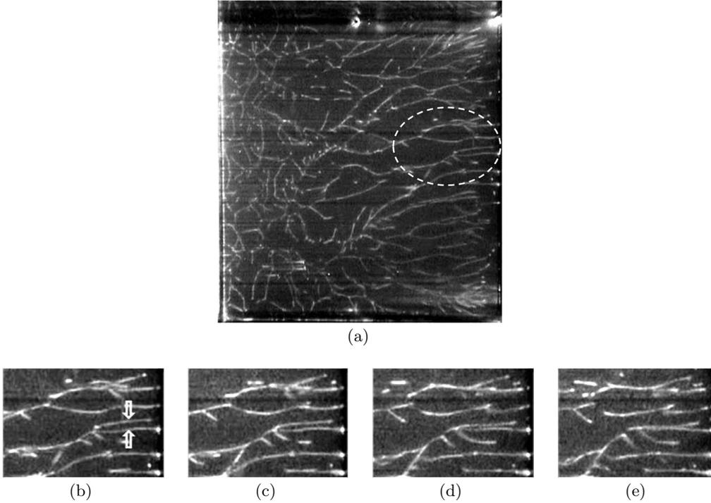
FIGURE 7. Dynamics of plumes observed by Puthenveettil & Arakeri (2005) at  $Sc = 600$  and  $Ra_w = 2.034 \times 10^{11}$ ; (a), The instantaneous planform of the entire convection surface of the cell of size  $87\text{mm} \times 98\text{mm}$ ; (b) to (e), zoomed views of size  $34\text{mm} \times 23\text{mm}$  of the merging plumes in the region showed by the dashed ellipse in (a) at the following different times; (b),  $t=0$  s; (c),  $t=4$  s; (d),  $t=8$  s; and (e),  $t=11$  s.
