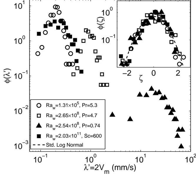
FIGURE 20. Distribution of merging velocity of plumes ( $V_m$ ) for different  $Ra_w$  and  $Pr$ . The inset shows the data in the main figure plotted as the pdf of the logarithm of the dimensionless merging velocities in their standardised form  $\zeta = (\ln(V_m/\overline{V_m}) - \ln(\overline{V_m}/\overline{V_m}))/\sigma \ln(\overline{V_m}/\overline{V_m})$ .
