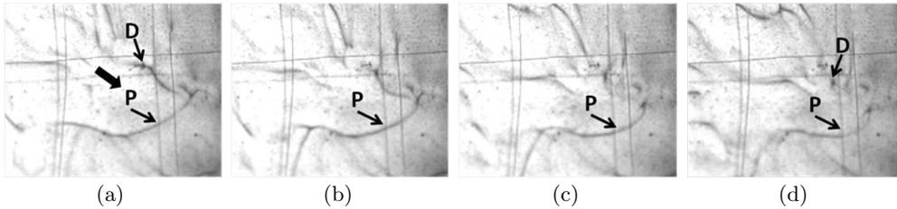
FIGURE 11. (a) to (d), Lateral motion of plumes due to shear at  $Pr = 4.7$ , and  $Ra_w = 2.65 \times 10^8$ . The plume P moves laterally along the direction of shear, identified by the motion of the feature marked by D. The images are of size  $98\text{mm} \times 79\text{mm}$  and separated by 2 s.
