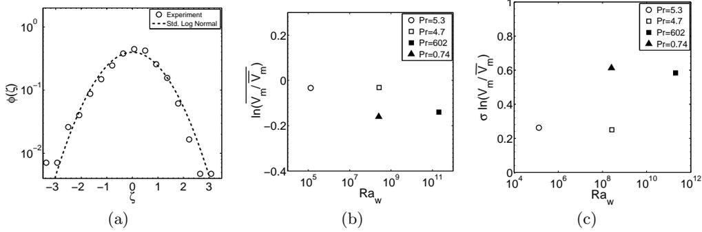
FIGURE 21. (a), The common probability density function of the logarithm of the dimensionless plume merging velocities in their standardised form  $\zeta = (\ln(V_m/\overline{V}_m) - \ln(\overline{V}_m/\overline{V}_m))/\sigma \ln(V_m/\overline{V}_m)$  at all  $Ra_w$  and  $Pr$ ; (b), Variation of the mean of the logarithm of the dimensionless plume merging velocities with  $Ra_w$ ; (c), Variation of the standard deviation of the logarithm of the dimensionless plume merging velocities
