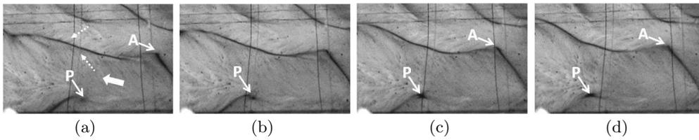
FIGURE 9. Dynamics of initiation and elongation of line plumes at  $Pr = 4.7$ , and  $Ra_w = 2.65 \times 10^8$ . Point P shows the location of initiation. The dashed arrows show the direction of motion in the boundary layers between the plumes. The images are of size  $98\text{mm} \times 65\text{mm}$  and are separated by 1.5 s.
