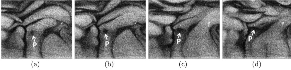
FIGURE 8. Sequence of images showing the dynamics of initiation and elongation of line plumes at  $Ra_w = 2.54 \times 10^8$  and  $Pr = 0.74$ . The point P shows the initiation of a line plume. The images are of size  $171\text{mm} \times 135\text{mm}$  and are separated by 0.2 s.
