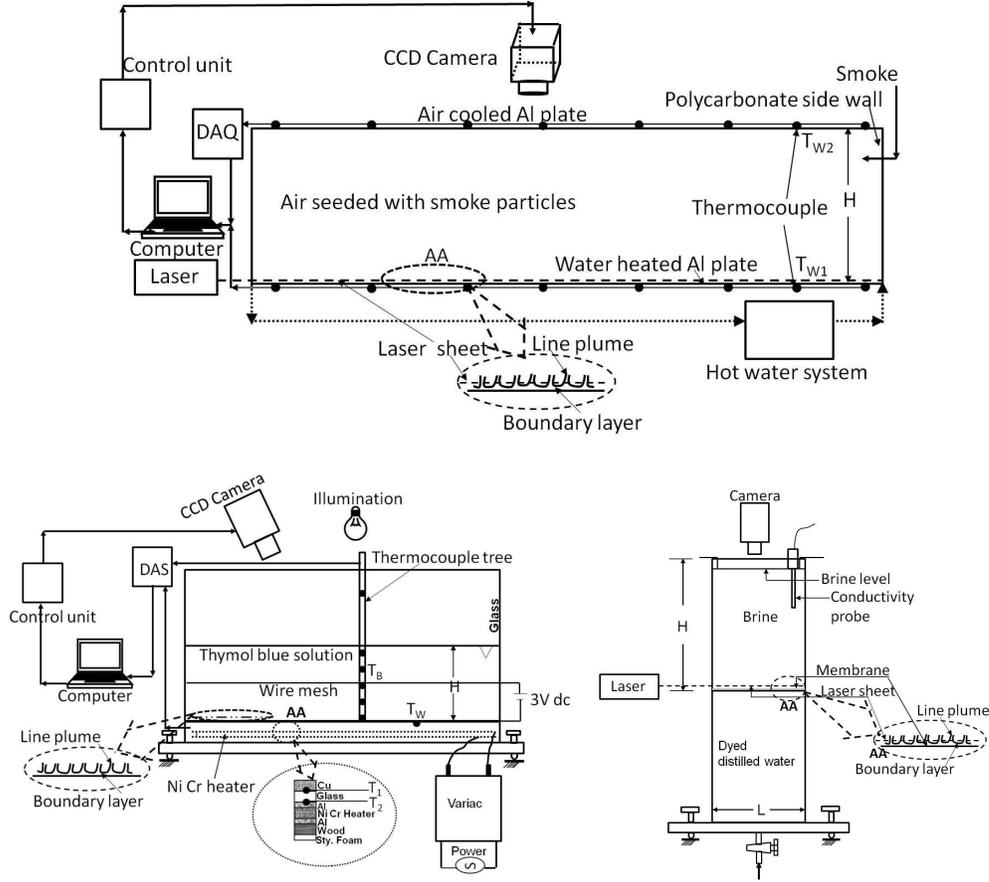
FIGURE 1. Schematic of the experimental setups used for studying; (a), steady temperature driven convection in air at  $Pr = 0.74$ ; (b), unsteady temperature driven convection in water at  $Pr = 3.6$  to  $5.3$  and (c), quasi-steady concentration driven convection at  $Sc = 602$  (Puthenveetil & Arakeri 2005).
