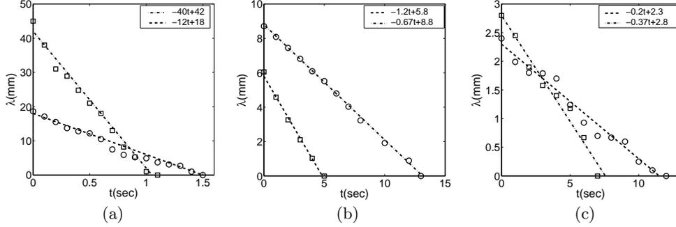
FIGURE 18. Measured variation of plume spacings ( $\lambda$ ) as a function of time ( $t$ ) in regions with shear ( $\circ$ ) and without shear ( $\square$ ) for; (a),  $Pr = 0.74$  at  $Ra_w = 2.54 \times 10^8$ ; (b),  $Pr = 4.7$  at  $Ra_w = 2.65 \times 10^8$  and; (c),  $Pr = 602$  at  $Ra_w = 2.034 \times 10^{11}$ .
