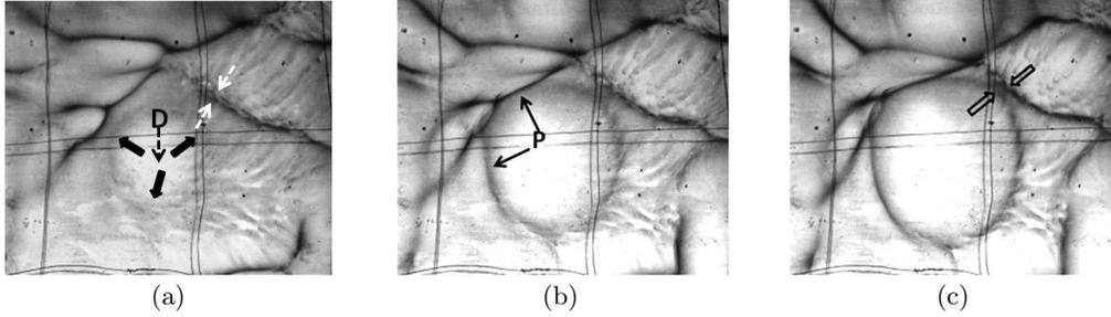
FIGURE 12. (a) to (d), Lateral plume motion due to local impingement of bulk flow at  $Pr = 5.3$ , and  $Ra_w = 1.31 \times 10^5$ . The filled arrows show the shear due to the downflow at D. The plumes P align at the outer periphery of the local shear. The dashed arrows show the direction of motion in the boundary layers between the plumes. The images are of size  $157\text{mm} \times 135\text{mm}$  and are at times 0 s, 8 s and 14 s respectively.
