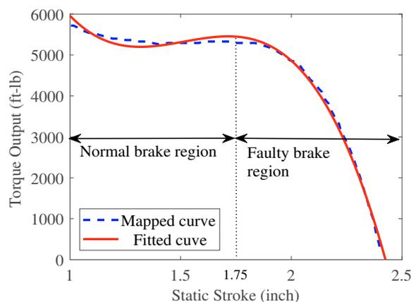
Fig. 1. Variation of brake torque with pushrod stroke for a type 20 brake chamber (Dunn et al. (2012))
