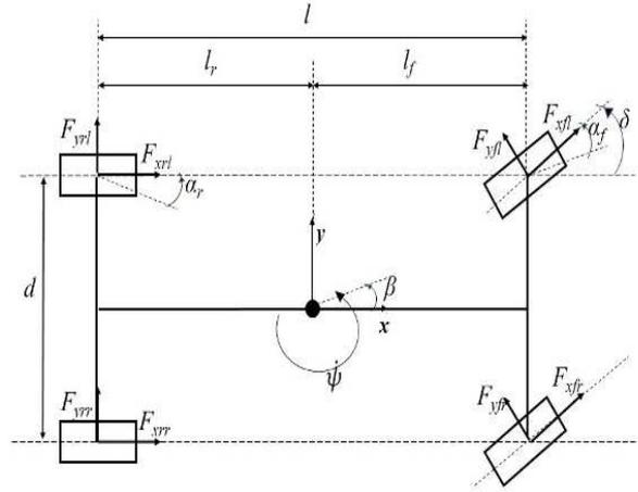
Fig. 2. Two-track model of a vehicle performing a left turn the distances of the front tire and the rear tire respectively from the CG of the vehicle.  $m_s$  and  $h_s$  are the sprung mass of the vehicle and the height of CG of sprung mass from the roll axis respectively.  $\psi(t)$ ,  $\phi_s(t)$ ,  $\delta(t)$ , and  $\beta(t)$  are yaw angle, roll angle, steering angle, and the vehicle side slip angle respectively.
