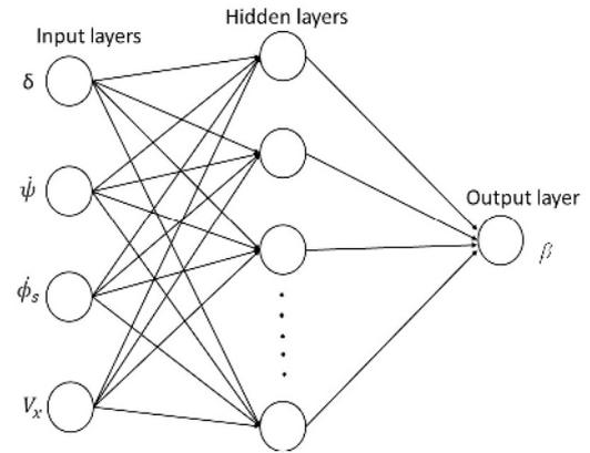
Fig. 4. ANN model for side slip angle estimation
