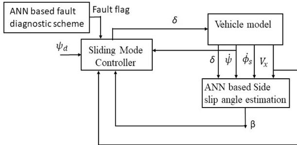
Fig. 3. Overview of yaw angle correction controller
