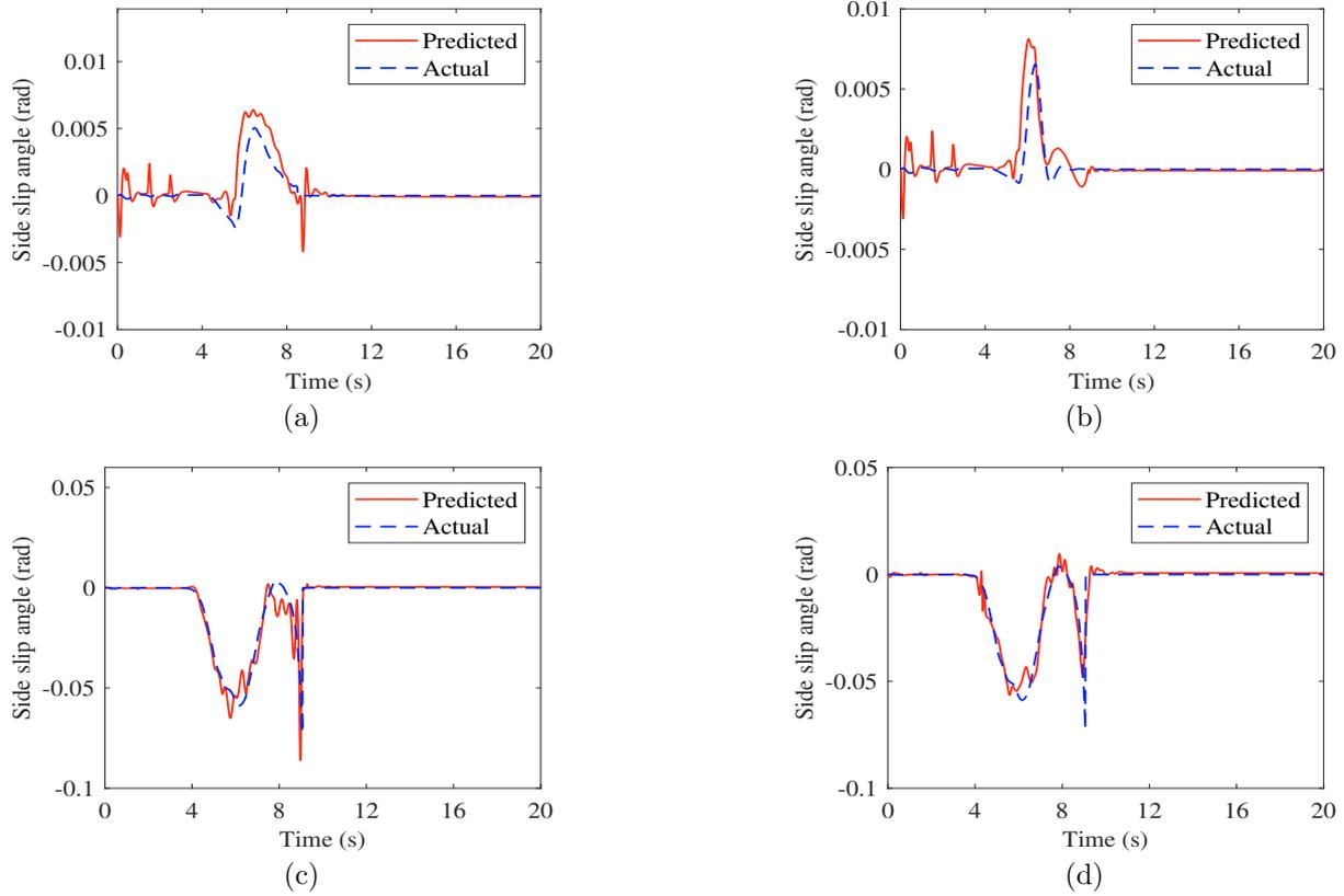
Fig. 5. Side slip angle estimation of a laden vehicle under full brake application with fault on front right brake: (a) Straight line maneuver with fault (15 % torque reduction), (b) Straight line maneuver with fault (25 % torque reduction), (c) Steady state circle maneuver with fault (15 % torque reduction), (d) Steady state circle maneuver with fault (25 % torque reduction)
