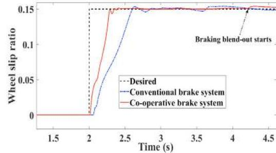
Fig. 8. Comparison of co-operative braking and conventional braking with PRERL
