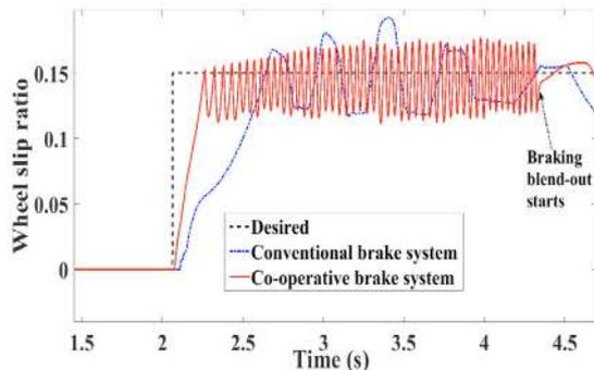
Fig. 7. Comparison of co-operative braking and conventional braking with CRL
