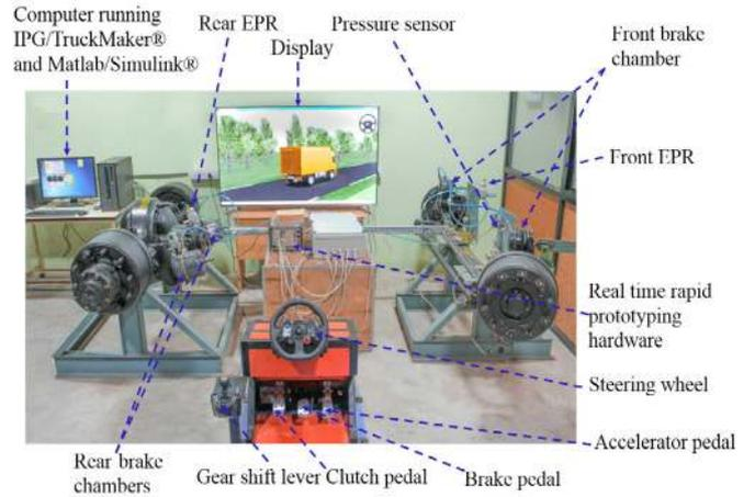
Fig. 6. Hardware-in-Loop brake system experimental setup
