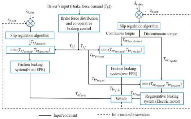
Fig. 5. Proposed co-operative braking control
