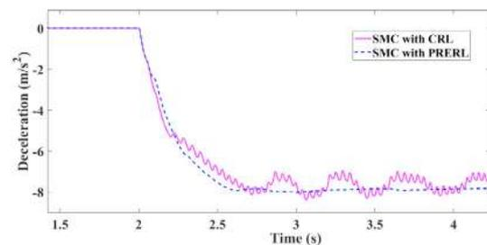
Fig. 9. Comparison of deceleration with CRL and PRERL during co-operative braking
