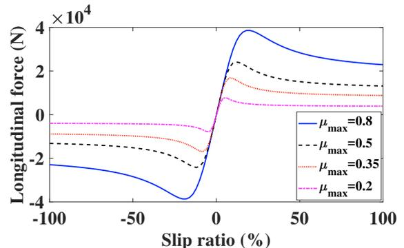
Fig. 4. Longitudinal tire characteristic curve
