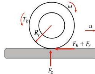
Fig. 3. Forces acting on the wheel during longitudinal motion
