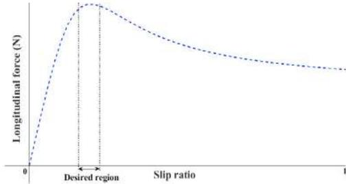
Fig. 2. Longitudinal force Vs Slip ratio
