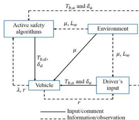
Fig. 1. Vehicle's active safety system layout
