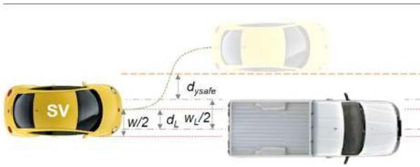
Fig. 3. Desired Lateral Position
