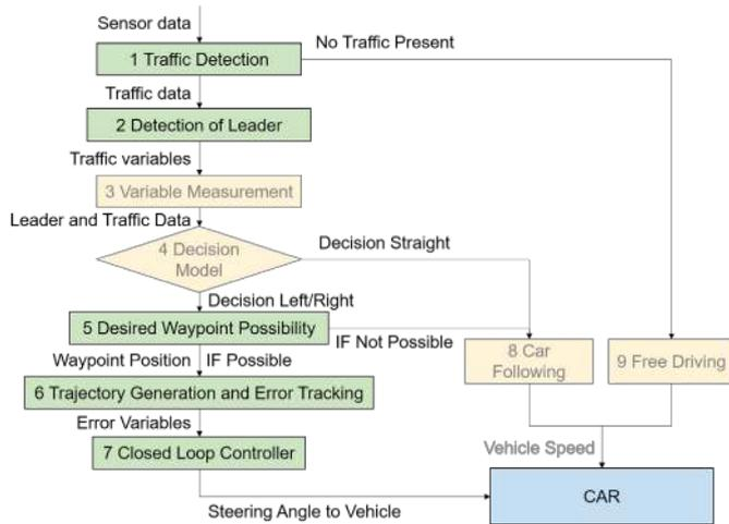
Fig. 1. Overview of the vehicle motion model
