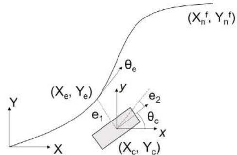
Fig. 5. Trajectory coordinates for error tracking
