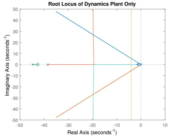
Fig. 6. Root locus of transfer function from  $\delta$  to  $y_L$
