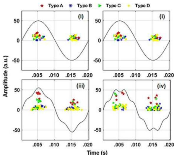
**Fig. 5** PRPD for sample types A, B, C and D for (i) fundamental frequency, (ii) 3f with 4% THD, (iii) 5f with 10% and (iv) 7f with 10% THD
