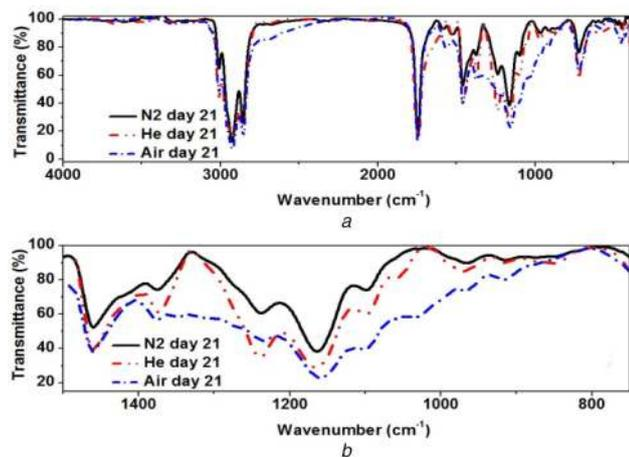
**Fig. 8** IR spectra of ester liquid on the 21st day under  $N_2$ , He and air medium of ageing (a) From 400 to 4000  $cm^{-1}$ , (b) From 700 to 1500  $cm^{-1}$
