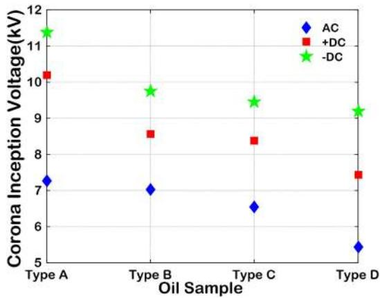
Fig. 2 Variation in CIV of Type A, Type B, Type C and Type D liquid under AC, +DC and -DC voltages
