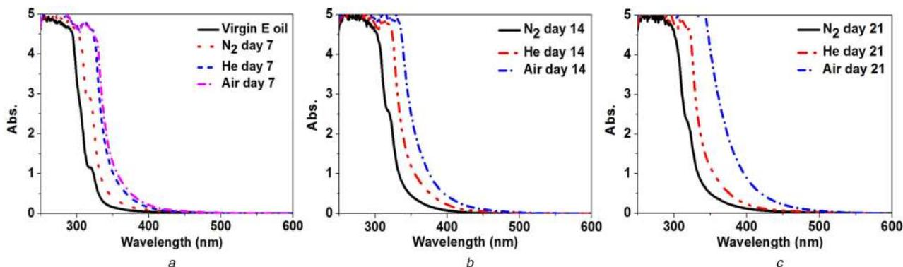
**Fig. 7** UV-Vis absorption spectra of ester liquid under  $N_2$ , He and air medium as on (a) Day 7, (b) Day 14, (c) Day 21
