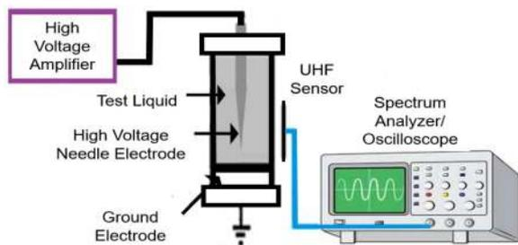
Fig. 1 Experimental setup for CIV measurement
