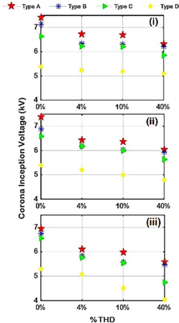
Fig. 3 Variation of CIV with respect to different THDs for oil samples for (i) 3f harmonics, (ii) 5f harmonics, and (iii) 7f harmonics
