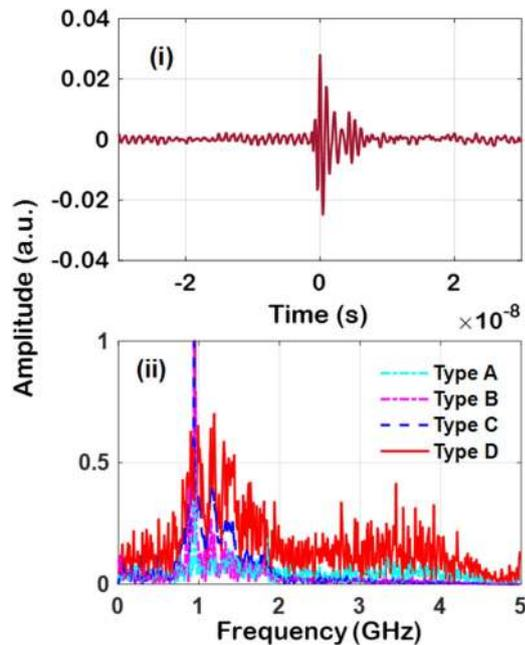
**Fig. 4** (i) Typical UHF signal formed due to corona activity in thermally aged ester liquid, (ii) FFT analysis of UHF signal formed due to corona discharge activity in different liquid samples
