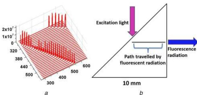
Fig. 10 Fluorescence measurement with different cuvette orientations
