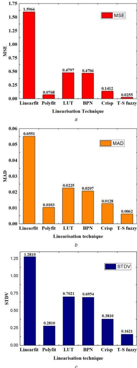
**Fig. 11** Graphical error analysis of IR sensor using (a) MSE, (b) MAD, (c) STDV
