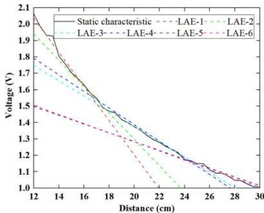
**Fig. 9** IR sensor static characteristic
