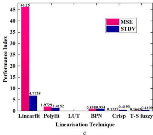
**Fig. 6** Performance comparison using different LTs for thermistor linearisation
