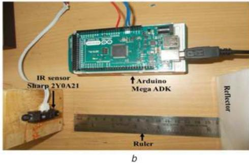
**Fig. 8** Real-time environment of IR sensor
