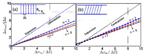
FIG. 4. Ladder networks with multiple identical bypasses: (a) Vertical bypasses (b) Forward slants.  $R_d/R_b = 3$ ,  $R_d/R_e = 2$ ,  $R_d = 1.5\text{kg}/\text{mm}^4\text{s}$  and  $\beta = 1.4$ .
