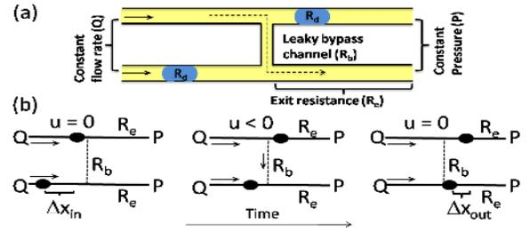
FIG. 1. (a) Ladder with a vertical bypass (b) Three distinct configurations are possible when a pair of drops traverse through a symmetric ladder network; Black objects represent drops. Full and dashed lines denote transport and bypass channels respectively. Arrows show flow direction.
