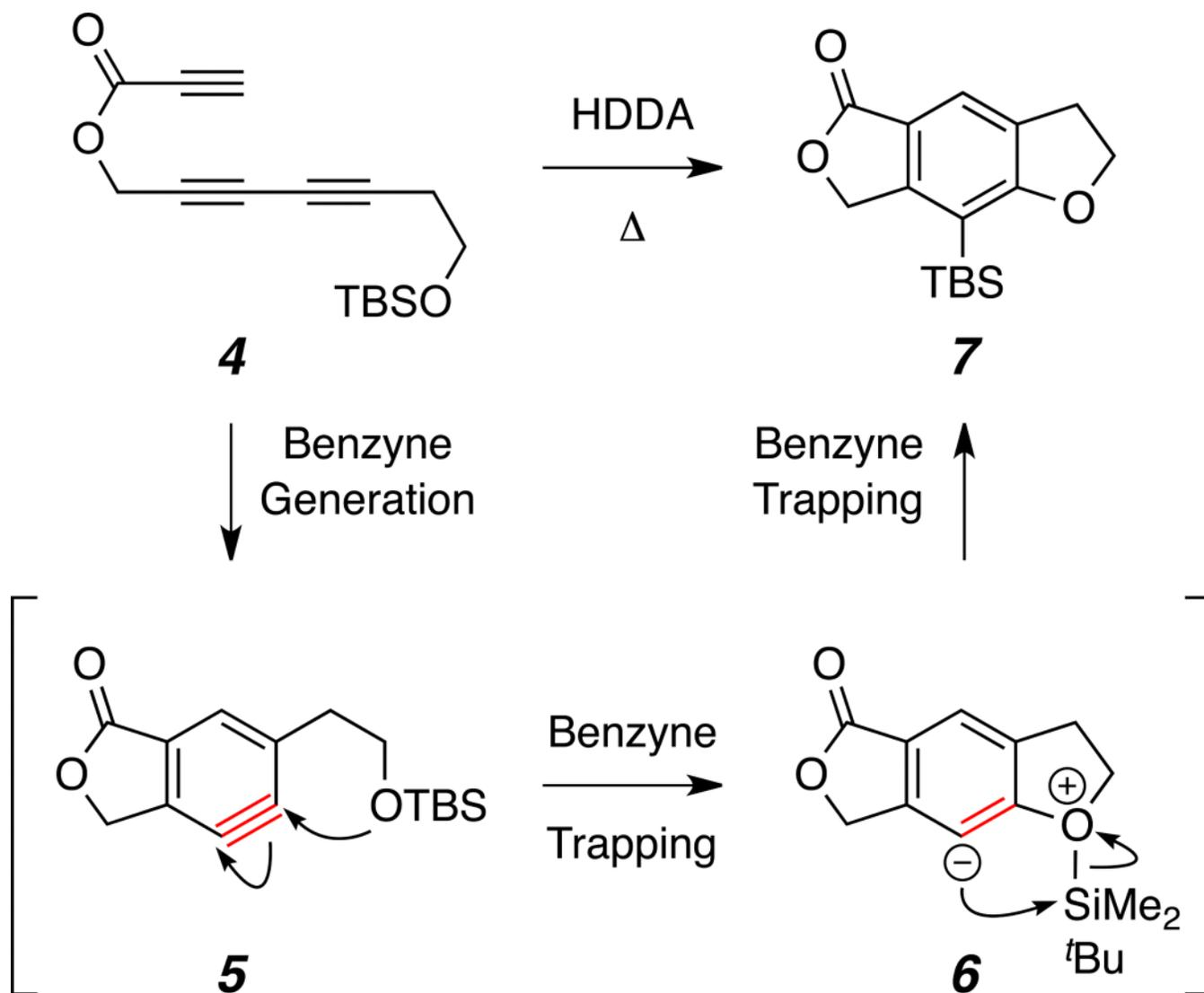
**Figure 2.** Intermediates involved (benzyne **5** and zwitterion **6**) in the HDDDA cascade conversion of triyne **4** to phthalide **7**. TBS: *t*-butyldimethylsilyl.
