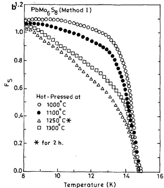
Fig. 6a, b. The specific heat jump (a), and the  $T_C$  distribution (b) of hot-pressed samples
