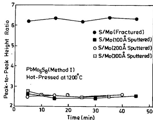
**Fig. 4.** Auger elemental composition ratios of one of the samples
