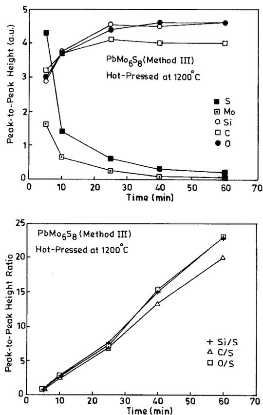
Fig. 2. Diffusion of impurities at the grain boundaries of sputtered (100 Å) sample
