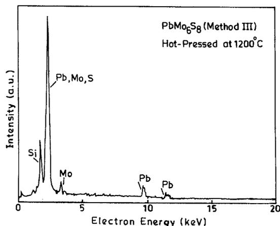
Fig. 1. EDX analysis of the sample prepared in a quartz tube
