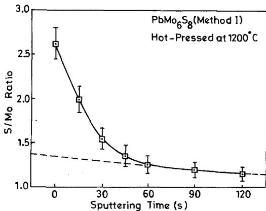
Fig. 7. Auger depth profiles of one of the samples
