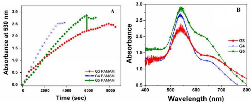
**Figure 5.** (A) Temporal response at 530 nm and (B) absorbance response obtained from U-bent POF probes functionalized with dendrimer of a different generation and thereafter, subjected to AuNP (OD 1.5).
