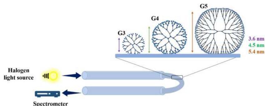
**Figure 1.** Schematic showing the experimental set-up with dendrimer-coated PMMA-POF coupled to a halogen light source and fiber optic spectrometer. Inset: PMMA surface modification with PAMAM dendrimer of different generations (G3, G4 and G5) and their dimensions explored in this study.
