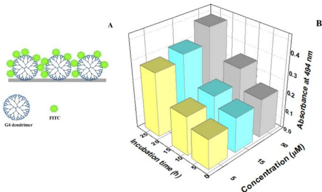
**Figure 3.** (A) Schematic representation of FITC binding to G4 PAMAM dendrimer on U-bent PMMA-POF probe surface and (B) saturated absorbance response at 494 nm of U-bent POF with varying incubation time and concentration of dendrimer solution (the probes were incubated in FITC solution of 0.1 mM concentration).
