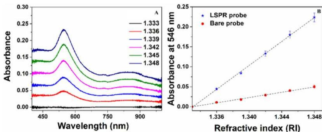
**Figure 6.** (A) Absorbance response and (B) RI sensitivity obtained from developed P-FOS subjected to sucrose solution of varying RI taking DI water as a reference.
