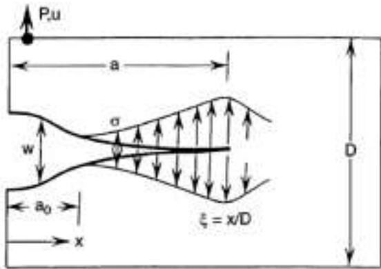
Fig. 8 – Cohesive crack and distribution of crack-bridging stresses.
