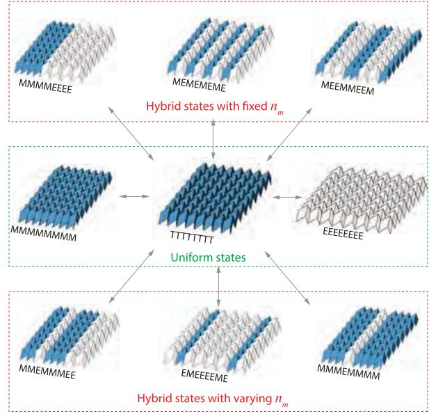
**Fig. 6 Realizations of the Morph pattern with 8x8 cells—the three uniform states and sample hybrid states. The double arrows indicate inter-transformability between states. *M*, *E*, *T* represent the strips in Miura mode, Eggbox mode, and Transition state, respectively. The parameter  $n_m$  is the number of strips in the Miura mode. The strips in the Eggbox mode are shown in white color.**
