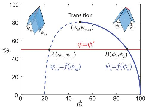
**Fig. 2 Configuration path of a Morph unit cell in terms of the folding angles. The Miura mode cells are represented by point A and the Eggbox mode cells are represented by point B which lie on the dashed and solid curves, respectively.**
