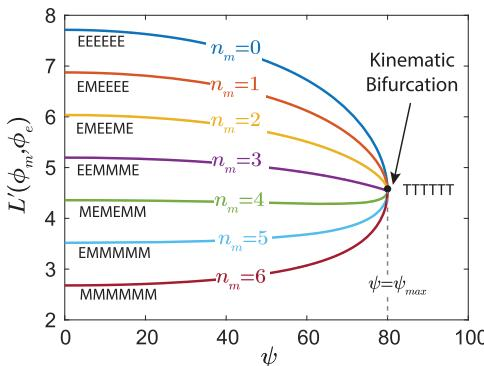
**Fig. 7 Kinematic branches of the Morph pattern.** *EEEEEEE*, *MMMMMM*, *TTTTTT* are uniform states and the rest are hybrid states. The parameter  $n_m$  denotes the number of strips in the Miura mode. The panel geometry was chosen as  $\alpha = 60$  deg,  $\beta = 40$  deg, and  $a = 1$ .
