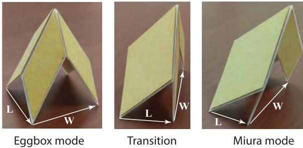
**Fig. 3 Physical model of the Morph unit cell**
