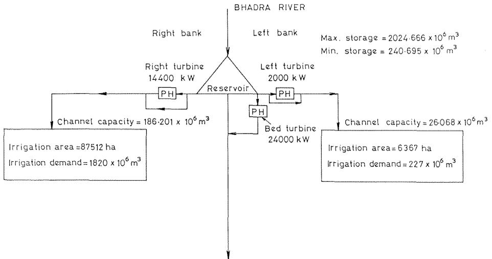
Fig. 1 Schematic diagram of Bhadra reservoir project.
