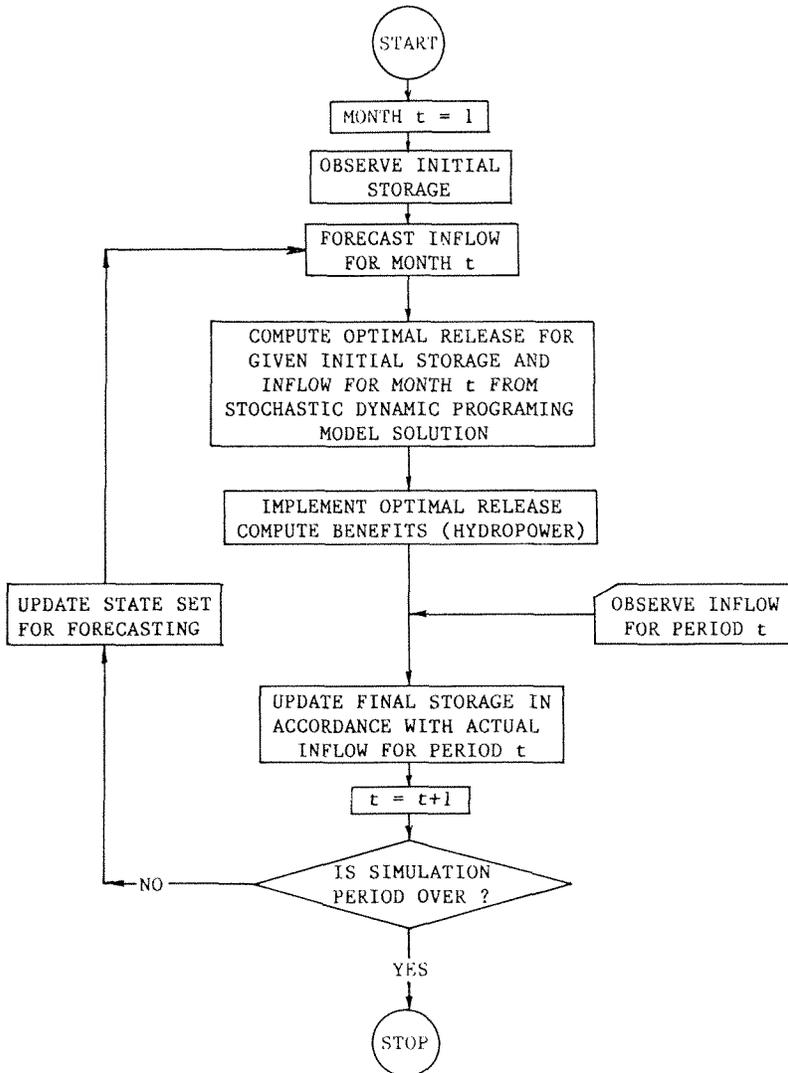
Fig. 2 Block diagram for real-time simulation.
