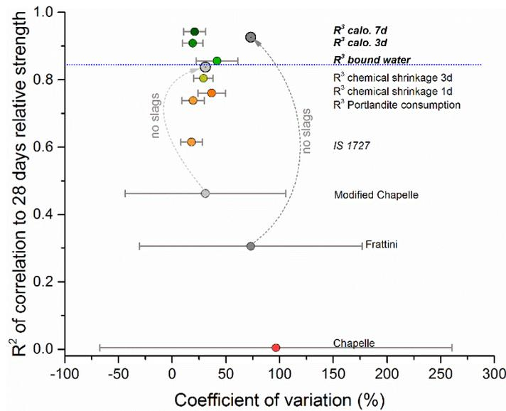
Figure 5 Correlation to 28 days relative strength vs. coefficient of variation (CV) plot, dotted blue line corresponds to  $R^2$  value equal to 0.85, dashed grey arrows indicate the improvement of the correlation for Frattini and Modified Chapelle tests by exclusion of the slag.
