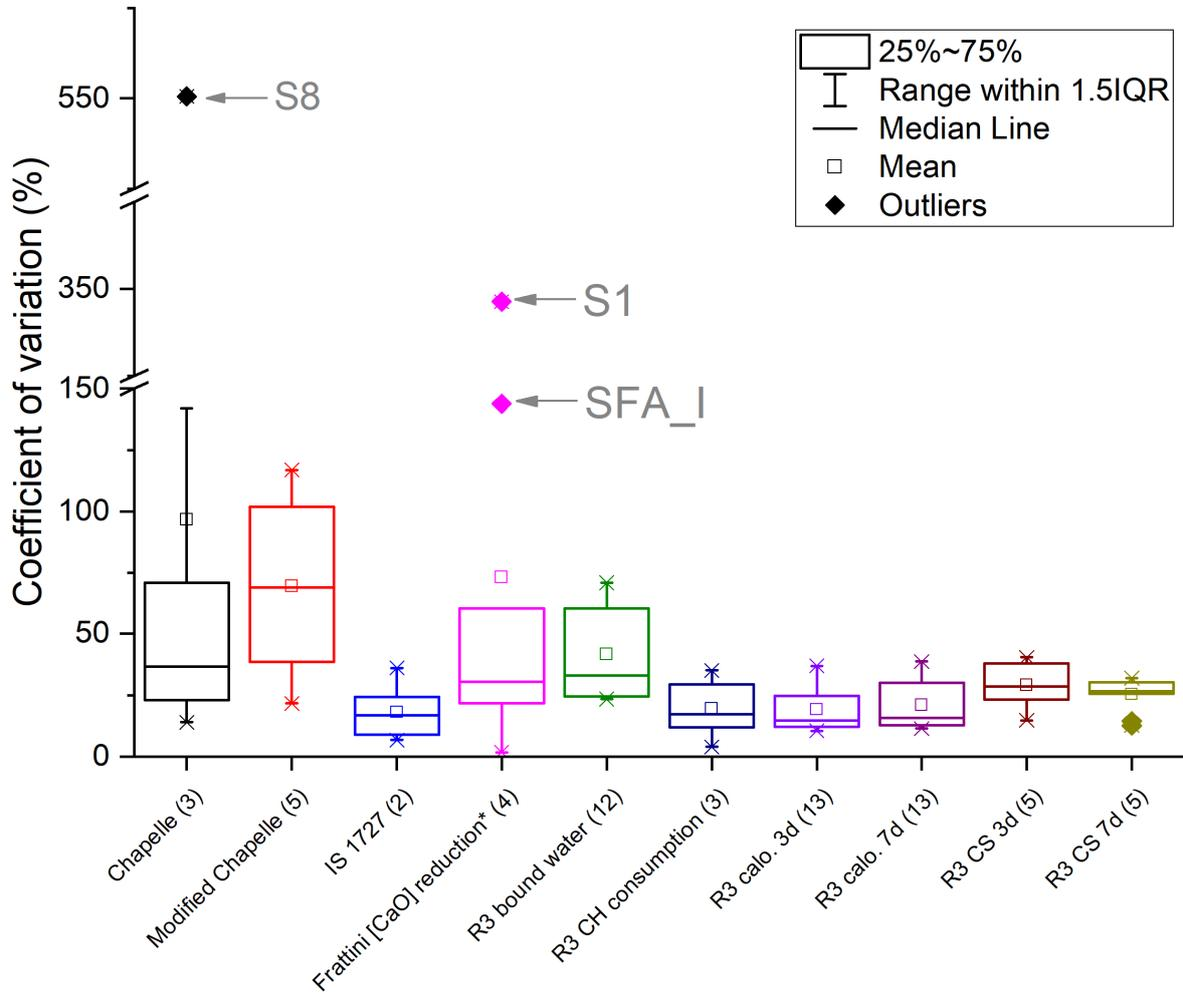
**Figure 4** Box chart for coefficient of variation (CV) for different methods, numbers in parentheses along the x-axis refer to the number of participants. R<sup>3</sup> CH consumption refers to portlandite consumption for R<sup>3</sup> model test; R<sup>3</sup> calo. 3d and R<sup>3</sup> CS 3d refer to calorimetry heat release and chemical shrinkage for the R<sup>3</sup> model, respectively.
