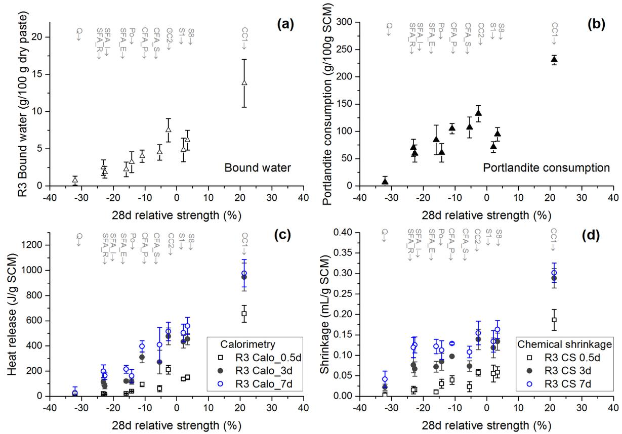
Figure 3 Plots of the  $R^3$  model test methods to 28 days relative strength, the SCMs corresponding to the points are labelled on top of each plot. (a) Bound water test, (b) Portlandite consumption, (c) Cumulative heat release for 0.5, 3 and 7 days and (d) Chemical shrinkage at 0.5, 3 and 7 days. Average values are shown by symbols, the error bars represent  $1\sigma$ .
