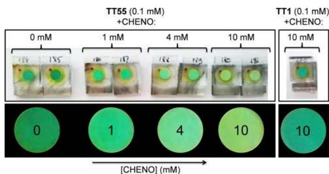
**Figure 3.** Top: pictures of the DSSC devices made with **TT55** (0.1 mM in THF) and different concentration of CHENO (0, 1, 4, and 10 mM in THF) adsorbed on [9+4]  $\mu\text{m}$  thick films; the benchmark device made with the carboxyl-substituted dye **TT1** (0.1 mM) in EtOH with 10 mM of CHENO is shown for comparison purpose. Bottom: Enlargement of the active area.
