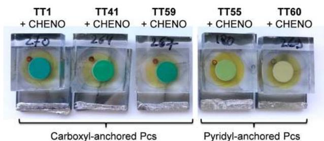
**Figure 2.** Pictures of the DSSC devices made with dyes **TT1**, **TT41**, **TT59**, **TT55** and **TT60** adsorbed on [9+4]  $\mu\text{m}$  thick films; dye solutions were prepared at a concentration of 0.1 mM of Pc and 10 mM of CHENO in THF (except for **TT1** in EtOH).
