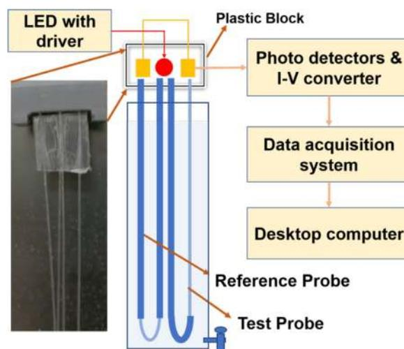
**Fig. 1.** Schematic showing block diagram of experimental setup consists of two U-bent POFs (decladded region of fiber represented as a thin line) dipped in a 55 cm long liquid column, home-made plastic block to house LED and PDs, optoelectronic circuitry, and DAQ.
