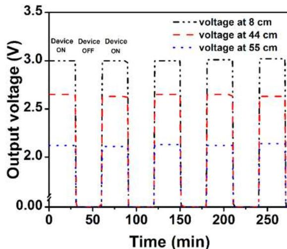
**Fig. 5.** Temporal response of the sensor over four hours indicating a stable response. The sensor was switched 'ON' for 30 min and then switched 'OFF' for the next 30 min at different liquid levels.
