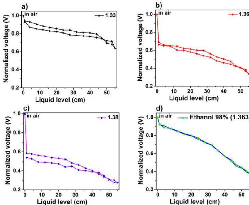
**Fig. 3.** Normalized differential voltage response from the fiberoptic level sensor subjected to filling and draining of liquids of different refractive index values including salt solutions of RI (a) 1.33 (no salt), (b) 1.36 and (c) 1.38 as well as (d) ethanol 98% with RI value of 1.363.
