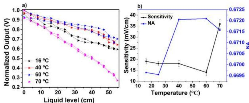
**Fig. 4.** (a) The relationship between normalized voltage and the liquid level with temperature various of 16 °C, 40 °C, 60 °C and 70 °C (b) The relationship between sensitivity vs temperature of 16 °C, 25 °C, 40 °C, 60 °C and 70 °C having sensitivity of 1.9, 1.8, 1.8, 1.4 and 3.6 mV/mm respectively.
