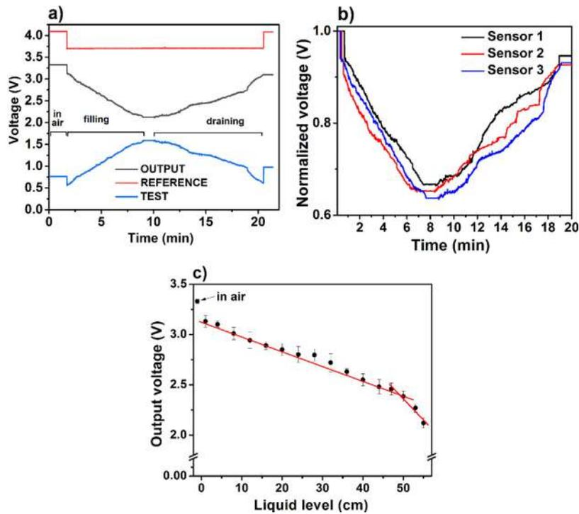
**Fig. 2.** (a) Sensor response recorded in terms of voltage while the 60 cm long glass column is continuously filled and drained with water over time of 20 min. (b) Normalized voltage response from three different test probes over time. (c) The relationship between output voltage and the liquid level.
