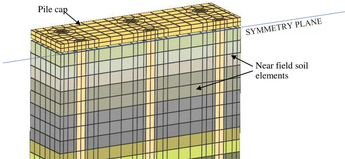
**Figure 3.** The finite element mesh of the pile group half model
