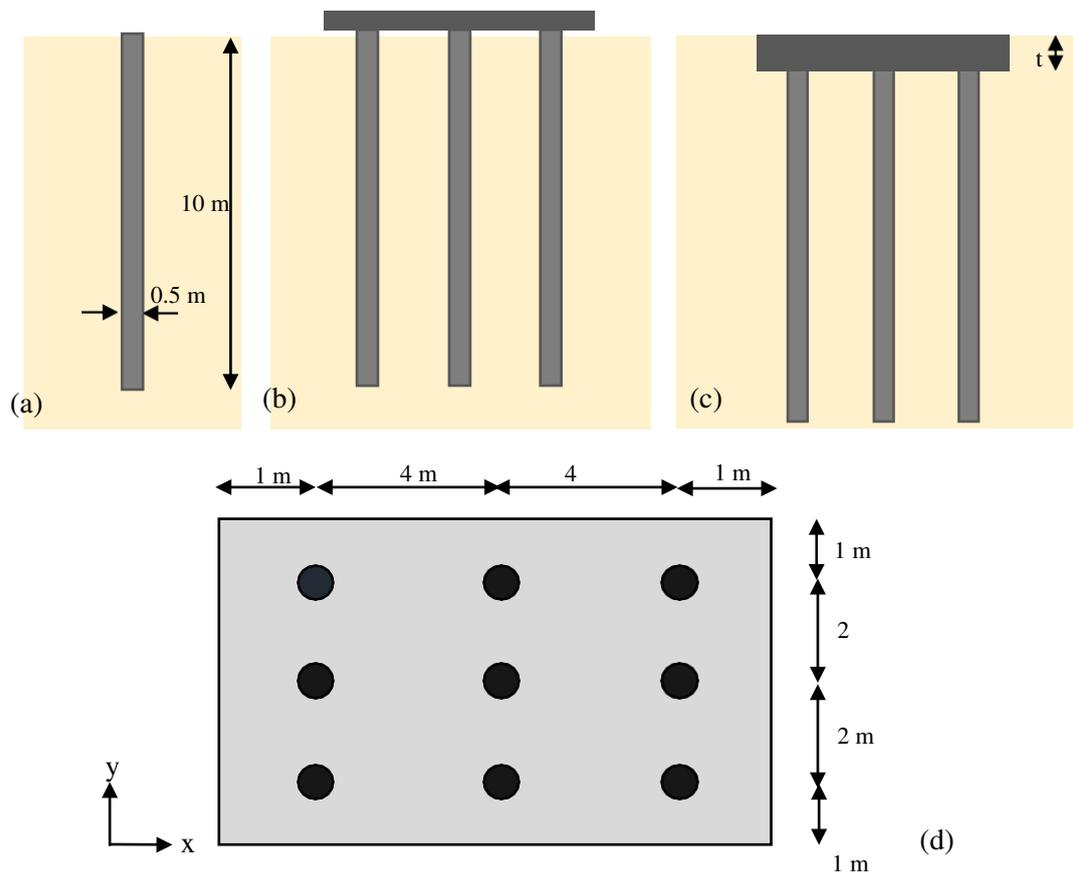
**Figure 2.** Schematic diagram showing (a) the single pile (b) pile group, (c) piled raft and (d) pile layout in PG and PR models
