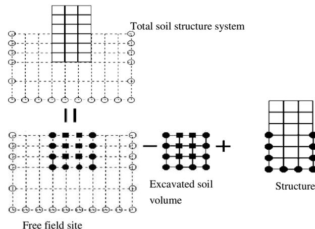
**Figure 1.** Partitioning of the total system into substructures in the Flexible Volume Method
