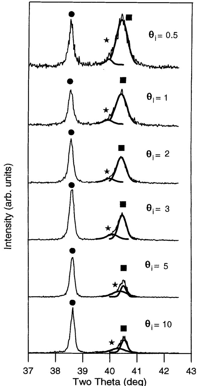
**Figure 4.** Partial GIXD scans of  $1 \times 10^{16}$  ions/cm $^2$   $N^+$  implanted Ti-6Al-4V alloy. (●,  $\alpha$ -Ti(0002); ★,  $\beta$ -Ti(110); ■,  $\alpha$ -Ti(1011)).
