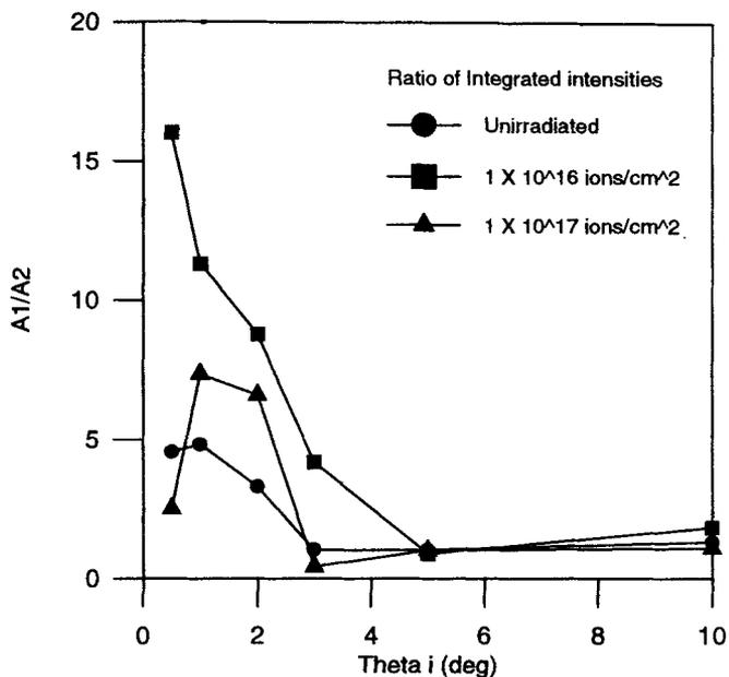
Figure 7. Ratio of integrated intensities A1/A2:  $I[\alpha\text{-Ti}(10\bar{1}1)]/I[\beta\text{-Ti}(110)]$ .
