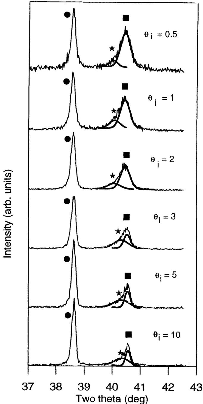
**Figure 3.** Partial GIXD scans of unirradiated Ti-6Al-4V alloy. (●,  $\alpha$ -Ti(0002); ★,  $\beta$ -Ti(110); ■,  $\alpha$ -Ti(1011)).
