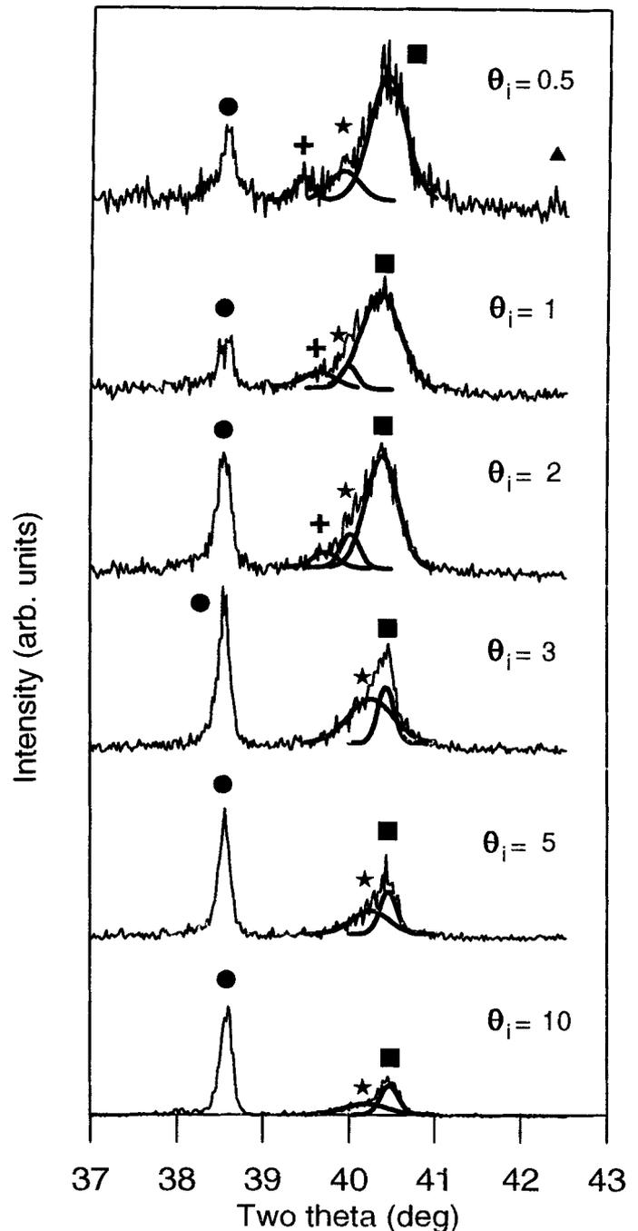
**Figure 6.** Partial GIXD scans of  $1 \times 10^{17}$  ions/cm<sup>2</sup> N<sup>+</sup> implanted Ti-6Al-4V alloy. (•,  $\alpha$ -Ti(0002); ★,  $\beta$ -Ti(110); ■,  $\alpha$ -Ti(1011); +,  $\epsilon$ -Ti<sub>2</sub>N(111); ▲,  $\delta$ -TiN(200)).
