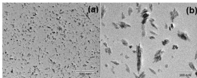
**Fig. 3** TEM picture of epoxy titania nanocomposites with different magnifications
