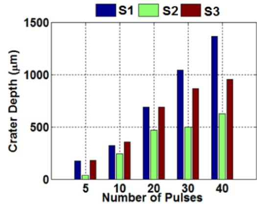
**Fig. 17** Variation of the depth of the crater with a number of laser pulses
