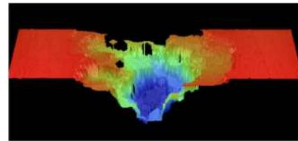
**Fig. 18** Typical 3D photograph of the crater formed by the laser pulse
