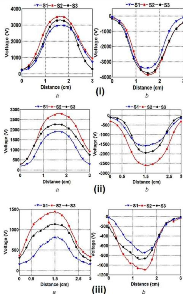
**Fig. 13** Variation in the potential distribution along the length of the epoxy specimen for (i) Virgin sample, (ii) 10 min corona-aged samples, (iii) 20 min corona-aged samples under (a) +DC, (b) -DC fields
