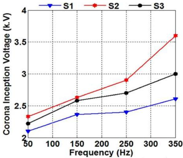
Fig. 6 Variation in CIV due water droplet with supply voltage frequency
