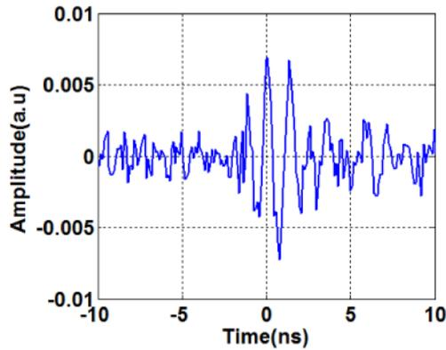
Fig. 14 Typical time domain representation of UHF signal generated during the inception
