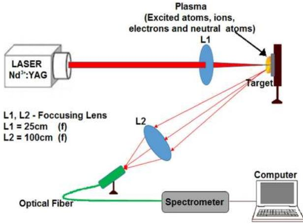
Fig. 5 LIBS experimental set-up
