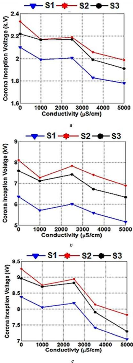
**Fig. 7** Variation in CIV with a conductivity of water droplet (a) AC, (b) +DC, (c) -DC
