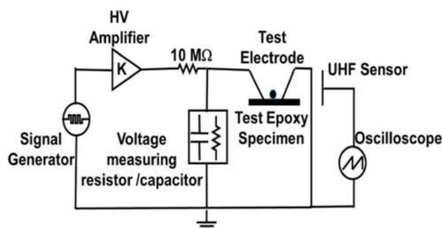
**Fig. 4** Experimental set-up for water droplet-initiated discharge studies
