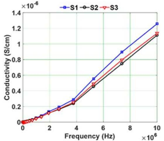
Fig. 11 Variation in conductivity of epoxy nanocomposites with frequency
