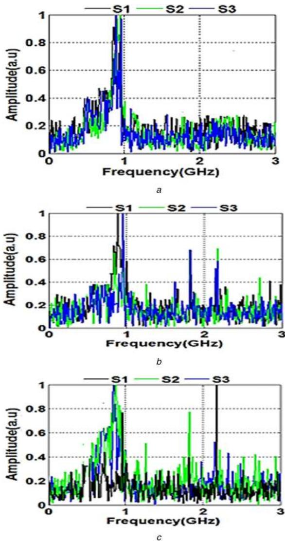
Fig. 15 FFT analysis of the inception voltages for all the samples S1, S2, and S3 under (a) AC field, (b) +DC field, (c) -DC field
