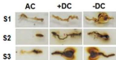
Fig. 10 Typical photograph of epoxy nanocomposites due to water droplet-initiated discharges under AC and DC voltages
