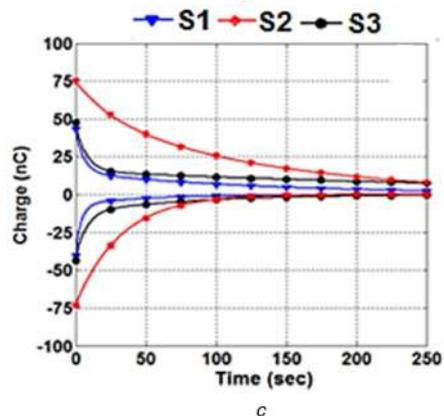
Fig. 12 Surface charge decay characteristics for (a) Virgin specimens, (b) 10 min corona-aged specimens, (c) 20 min corona-aged specimens under positive DC and negative DC corona charging
