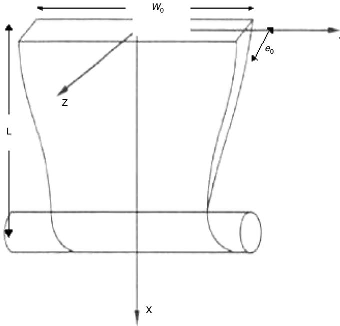
Fig. 1.1. Sketch of the geometry considered for the film casting process.
