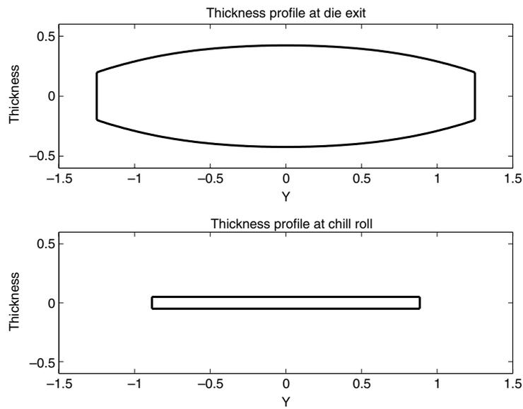
Fig. 4.5. Computed nozzle shape (top) and film thickness at take-up (bottom).
