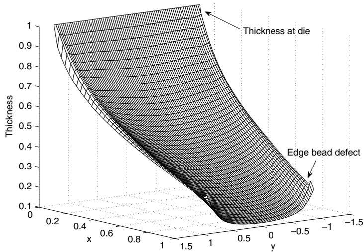
Fig. 1.2. Thickness profile of the film casting process with edge bead defect.
