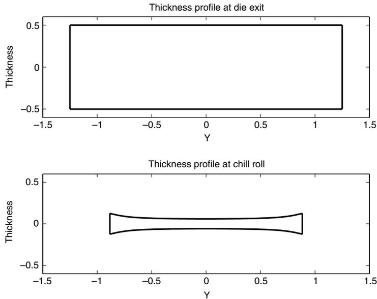
Fig. 4.4. Original nozzle shape (top) and computed film thickness at take-up (bottom).
