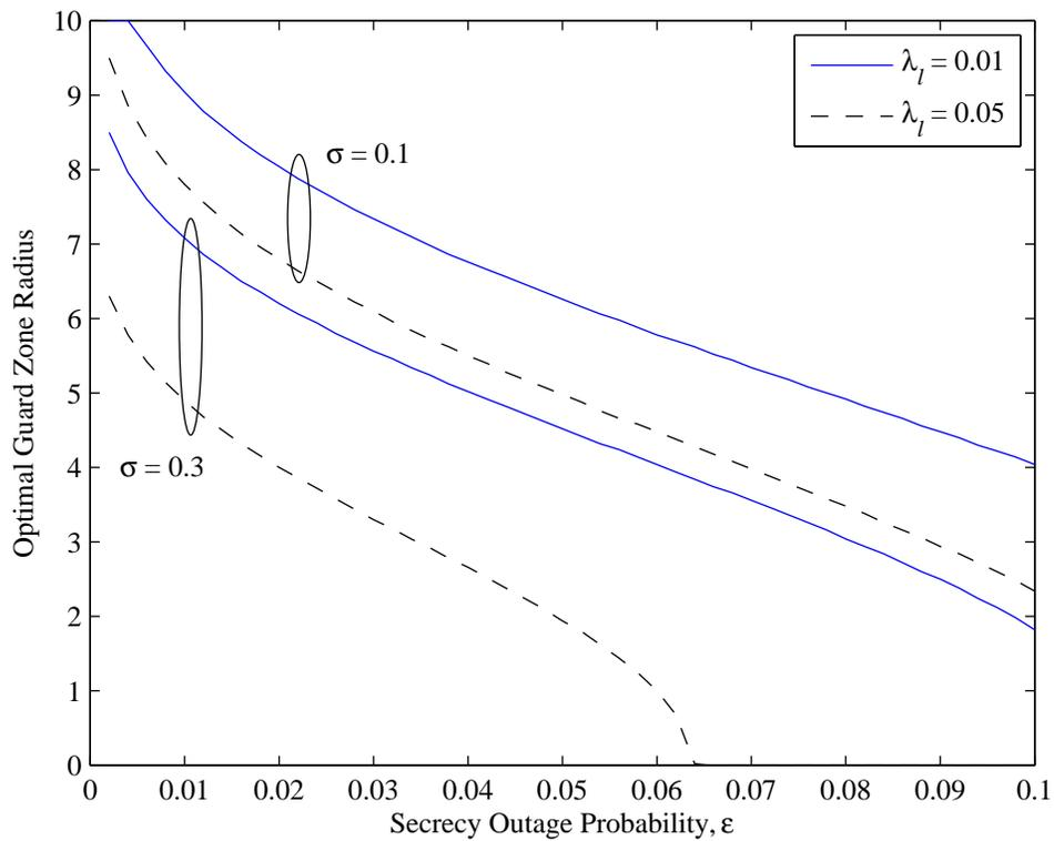
Fig. 7. The optimal secrecy guard zone radius versus the secrecy outage probability  $\epsilon$  for the case of cooperative transmitters. Results are shown for networks with different connection outage constraints, i.e.,  $\sigma = 0.1, 0.3$ , and different densities of legitimate transmitters, i.e.,  $\lambda_l = 0.01, 0.05$ . The other system parameters are  $r = 1$ ,  $\alpha = 4$ , and  $\lambda_e = 0.001$ .
