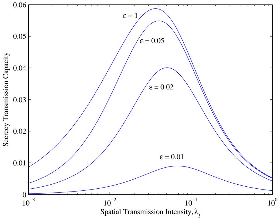
Fig. 3. The secrecy transmission capacity  $\tau^{\text{LB}}(r)$  in (20) versus the density of legitimate transmitters  $\lambda_l$ . Results are shown for networks with different secrecy outage constraints, i.e.,  $\epsilon = 0.01, 0.02, 0.05$ , as well as no secrecy constraint, i.e.,  $\epsilon = 1$ . The other system parameters are  $r = 1$ ,  $\alpha = 4$ ,  $\sigma = 0.3$ , and  $\lambda_e = 0.001$ .
