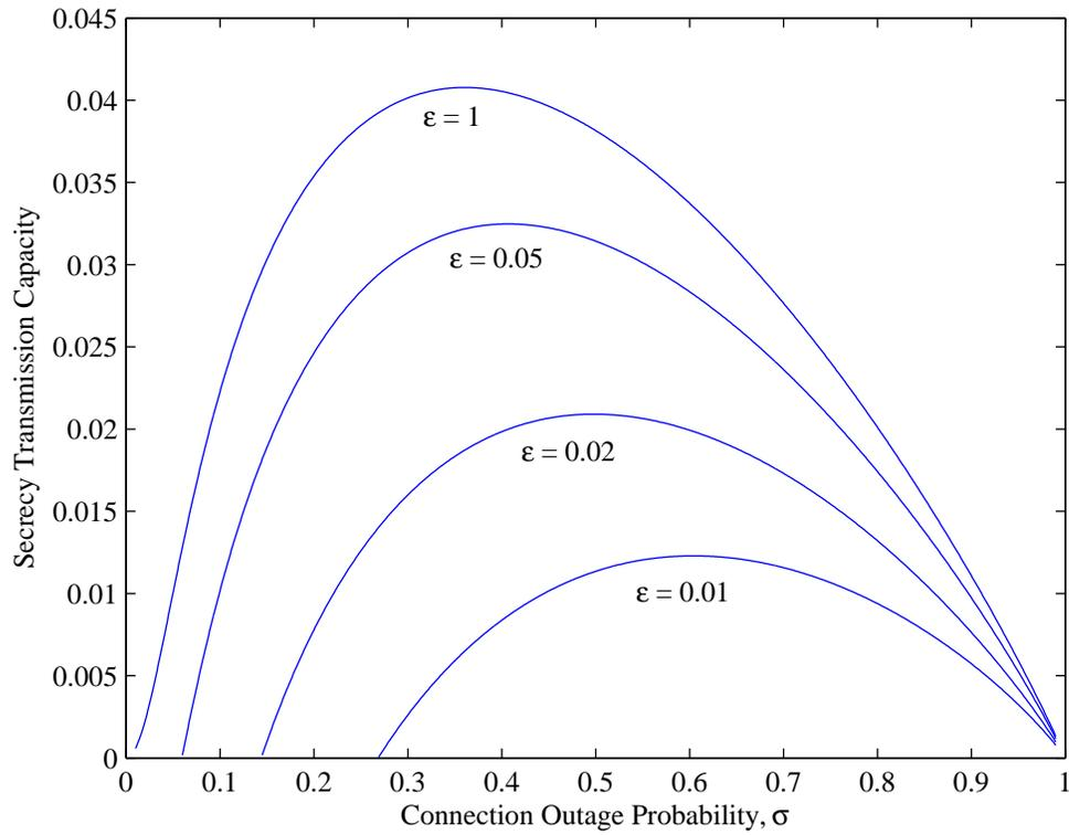
Fig. 4. The secrecy transmission capacity  $\tau^{\text{LB}}(r)$  in (20) versus the connection outage probability  $\sigma$ . Results are shown for networks with different secrecy outage constraints, i.e.,  $\epsilon = 0.01, 0.02, 0.05$ , as well as no secrecy constraint, i.e.,  $\epsilon = 1$ . The other system parameters are  $r = 1$ ,  $\alpha = 4$ ,  $\lambda_l = 0.01$ , and  $\lambda_e = 0.001$ .
