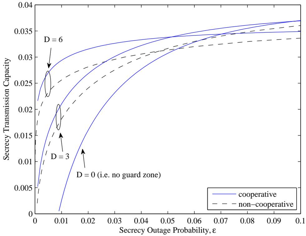
Fig. 5. The secrecy transmission capacity  $\tau^{\text{LB}}(r)$  with guard zone in (35) and (39) versus the secrecy outage probability  $\epsilon$ . Results are shown for networks with different guard zone radii, i.e.,  $D = 0, 3, 6$ . The other system parameters are  $r = 1$ ,  $\alpha = 4$ ,  $\sigma = 0.3$ ,  $\lambda_l = 0.01$ , and  $\lambda_e = 0.001$ .
