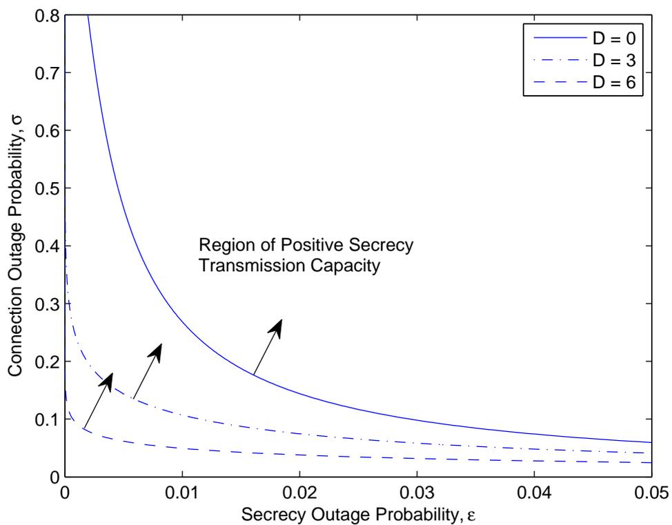
Fig. 6. The region of positive secrecy transmission capacity with and without secrecy guard zone. The case of cooperative transmitters is shown with different guard zone radii, i.e.,  $D = 0, 3, 6$ . The curves are plotted based on the relationship between the connection outage probability  $\sigma$  and the secrecy outage probability  $\epsilon$  given in (40). The other system parameters are  $r = 1$  and  $\lambda_e = 0.001$ .
