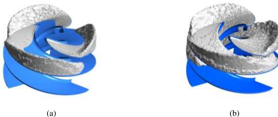
Figure 8. Cavity volume generated (time-averaged) in the inducer for (a) case 3A and (b) case 3B
