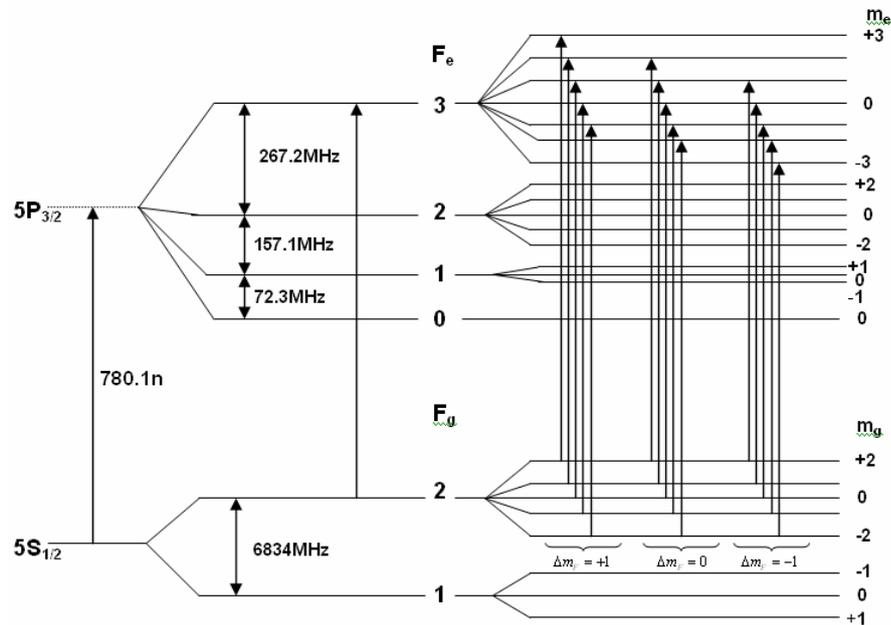
**Figure 1:** Energy level diagram for  $^{87}\text{Rb}$
