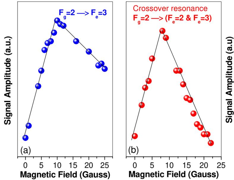
**Figure 4:** (a) Plot of signal amplitude versus magnetic field for the  $F_g=2$  to  $F_e=3$  transition. (b) Plot of signal amplitude versus magnetic field for the crossover line of  $F_g=2$  to  $F_e=2$  &  $F_e=3$ .
