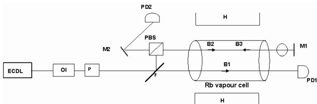
**Figure 2:** Schematic diagram of the experimental setup used. **Key:** ECDL-External Cavity Diode Laser, OI-Optical Isolator, F-Filter, PD -Photodiode, M-Mirror, PBS-Polarizing Beam Splitter, H-Helmholz coil, B1-Reference beam, B2-Pump beam, B3-Probe beam.
