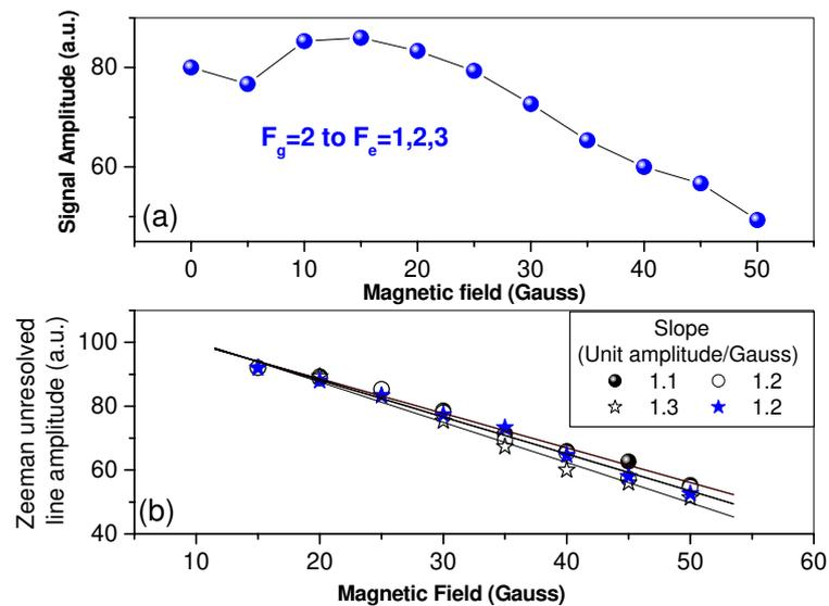
**Figure 5:** (a) Plot of signal amplitude versus magnetic field for unresolved Zeeman line from  $F_g=2$  to  $F_e=1, 2, 3$ . (b) Plot of signal amplitude versus magnetic field for unresolved Zeeman line from  $F_g=2$  to  $F_e=1, 2, 3$  above 10 gauss which is reproducibly linear.
