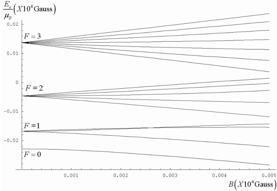
**Figure 6: (b)** Magnetic field dependence of  $^{87}\text{Rb}$  excited state ( $5P_{3/2}$ ) hyperfine energy levels.
