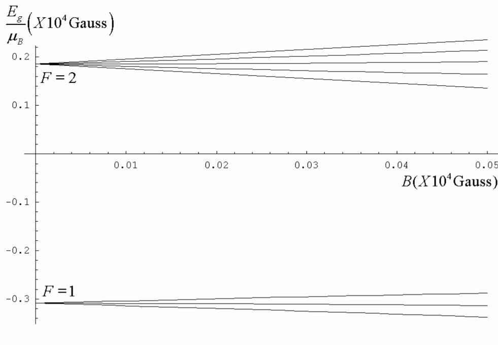
**Figure 6:** (a) Magnetic field dependence of  $^{87}\text{Rb}$  ground state ( $5S_{1/2}$ ) hyperfine energy levels.
