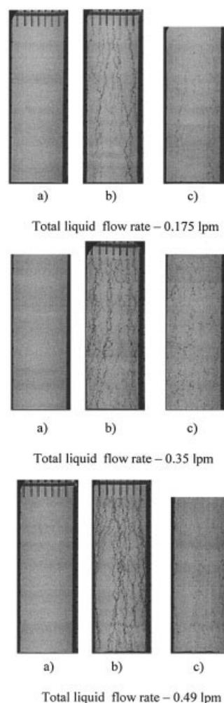
**Figure 4. X-ray images of bed in various conditions.**
