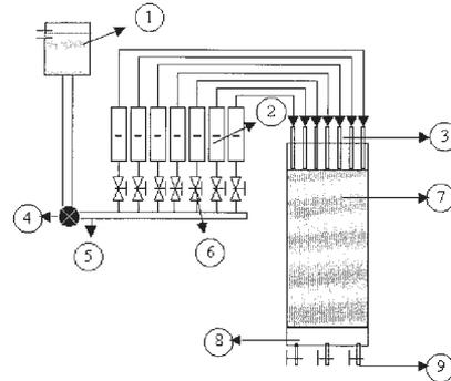
**Figure 2. Experimental arrangements for local holdup measurement.**
