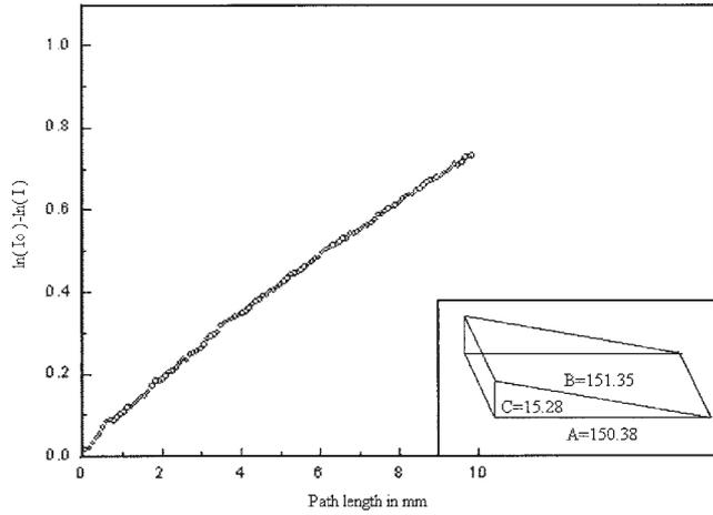
**Figure 1. Calibration graph for local/total liquid holdup measurement.**
