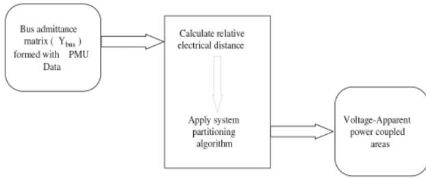
**Fig. 1** Scheme for partitioning the system into voltage–apparent power coupled areas
