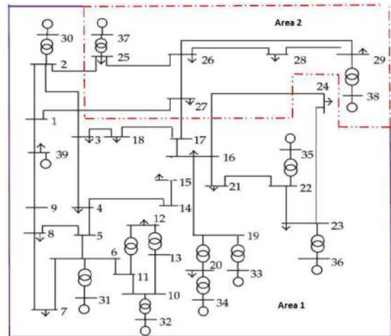
Fig. 6 Voltage-apparent power partitioning in New England 39-bus system-outage of line 15-16
