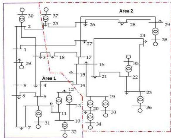
**Fig. 4** Voltage-apparent power partitioning in New England 39-bus system-base case
