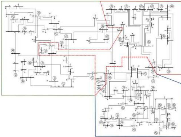
**Fig. 7** Voltage-apparent power partitioning in IEEE 118-bus system-base case
