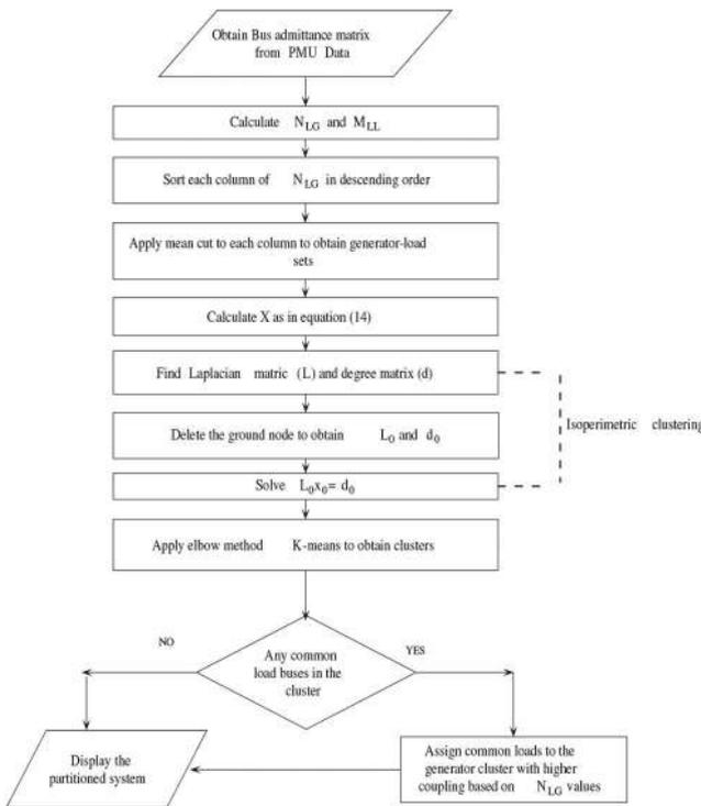
Fig. 2 Flowchart for partitioning system into voltage–apparent power coupled areas
