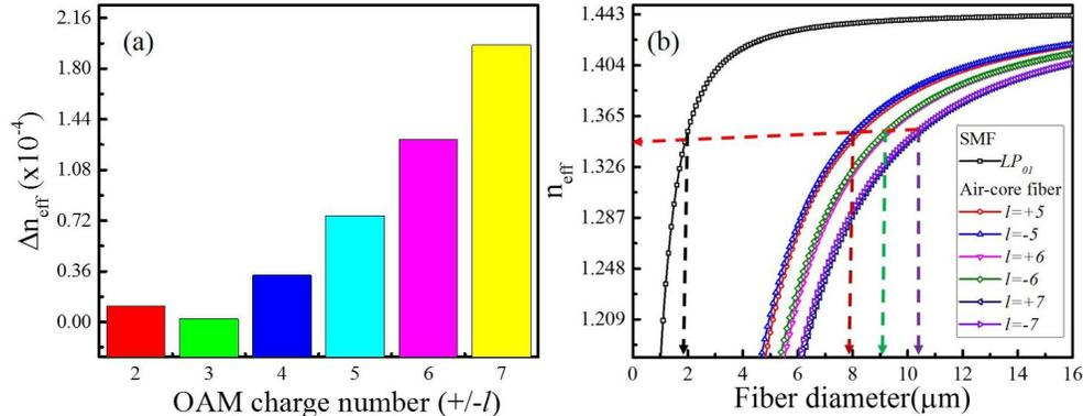
Figure 2 (a): The difference of effective index ( $\Delta n_{\text{eff}}$ ) of different OAM states in the selected air-core fiber and (b): Phase matching plot:  $n_{\text{eff}}$  of the  $LP_{01}$  mode in the SMF and that of the  $l = \pm 5, \pm 6$  and  $\pm 7$  modes in the air-core fiber are mapped as a function of fiber's diameter.
