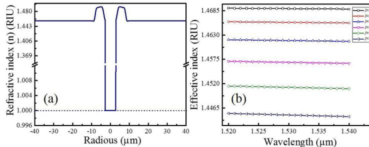
Figure 1 (a): The refractive index profile of the selected air-core fiber and (b): Effective index of OAM modes with different charge  $l$ -number
