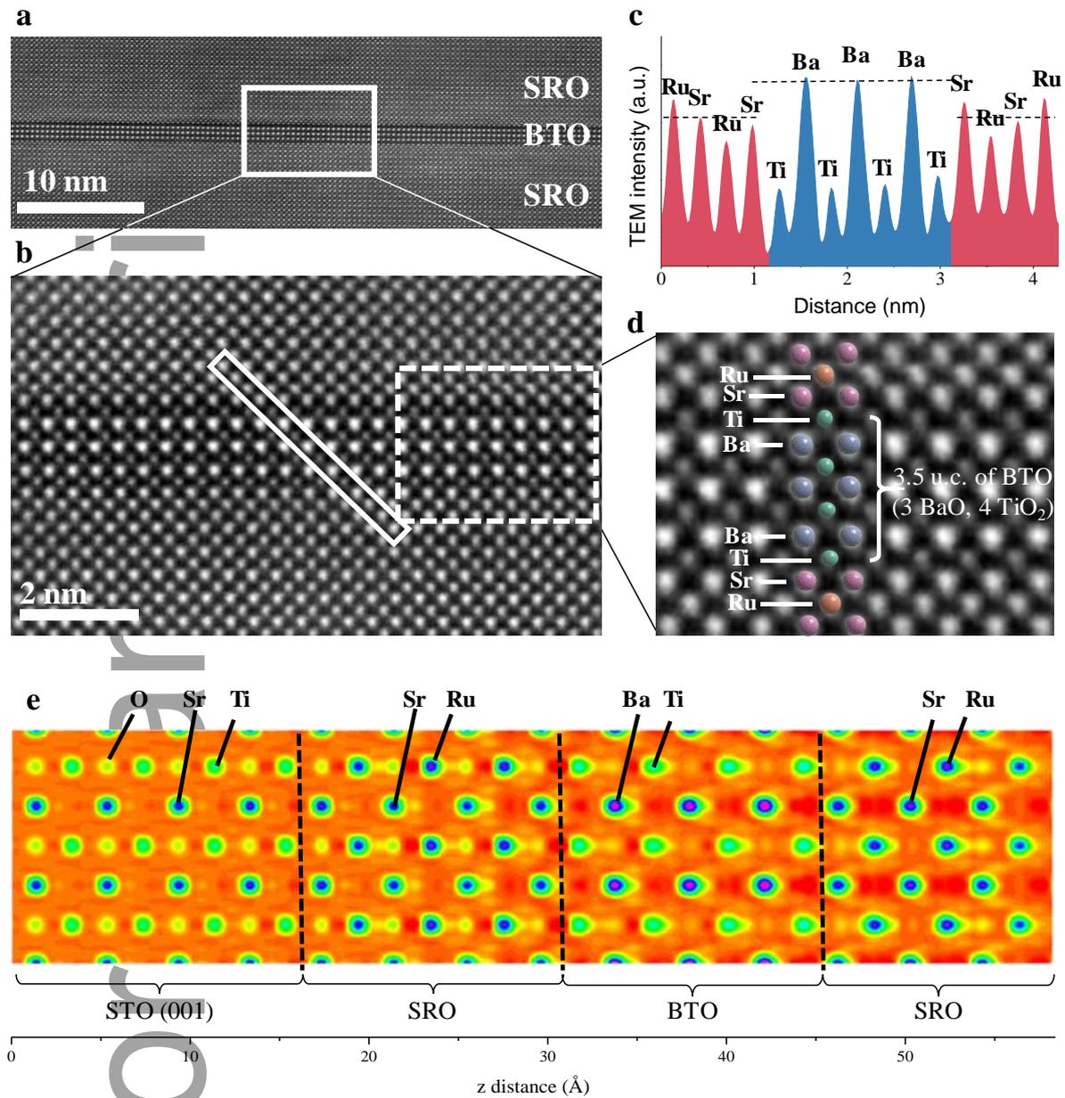
**Figure 2.** a) STEM image of the SRO/BTO/SRO heterostructure with  $P_{O_2} = 5$  mTorr. b) Magnified STEM image of the region inside the white box in 2a. c) Intensity line profile corresponding to the highlighted solid box in 2b. This profile clearly shows the TiO<sub>2</sub> termination at the top and bottom of the BTO layer. d) Magnified image of the area
