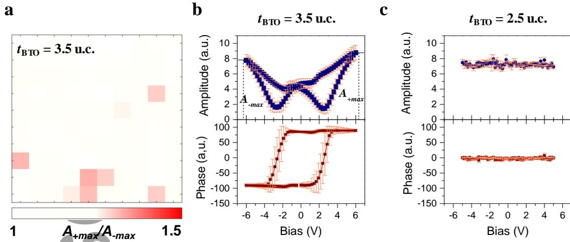
**Figure 3.** a) Color map of  $A_{+max}/A_{-max}$  for the SRO/BTO/SRO capacitor with  $t_{BTO} = 3.5$  u.c. and with  $P_{O_2} = 5$  mTorr. b) Averaged PFM amplitude and phase hysteresis loops measured at  $10 \times 10$  different positions in a single capacitor. The error bar indicates the standard deviation of the measured loops. c) Averaged PFM amplitude and phase hysteresis loops of the SRO/BTO/SRO capacitor with  $t_{BTO} = 2.5$  u.c..
