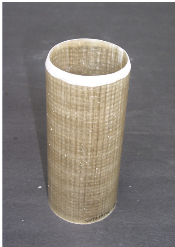
Fig. 3. Cylindrical shell with chamfered end.
