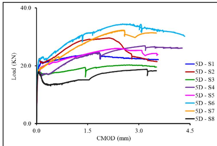
**Figure 5.1.** Load versus CMOD curves for specimens with 5D fibres (complete behaviour).
