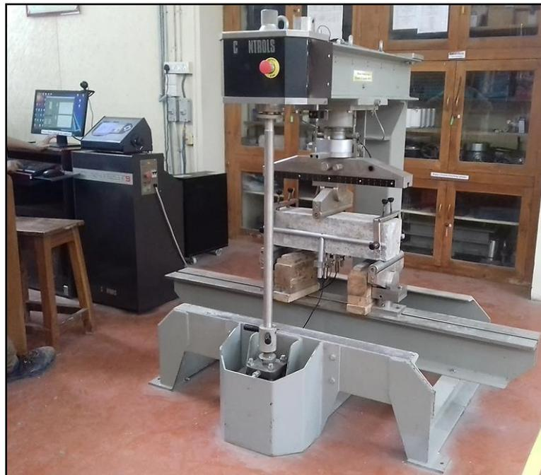
**Figure 2.** Test setup to determine flexural strength.
