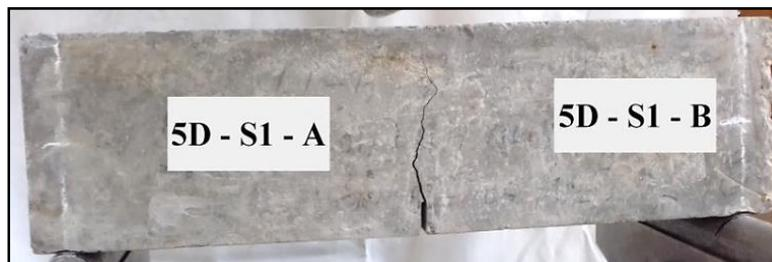
**Figure 3.** Typical failure pattern (shown for Specimen 5D - S1).
