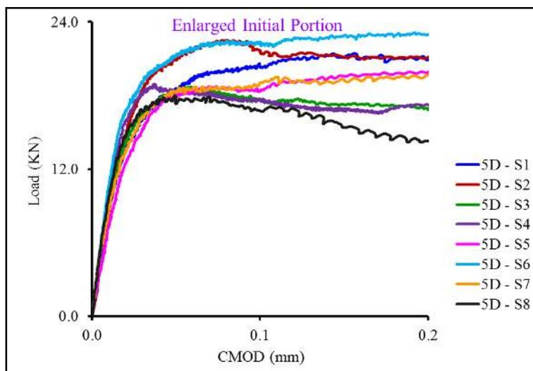
**Figure 5.2.** Load versus CMOD curves for specimens with 5D fibres (enlarged initial portion).
