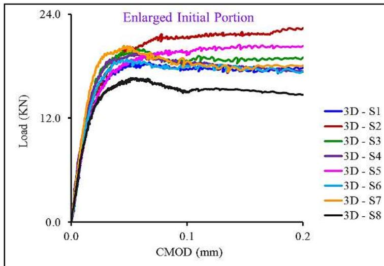
**Figure 4.2.** Load versus CMOD curves for specimens with 3D fibres (enlarged initial portion).
