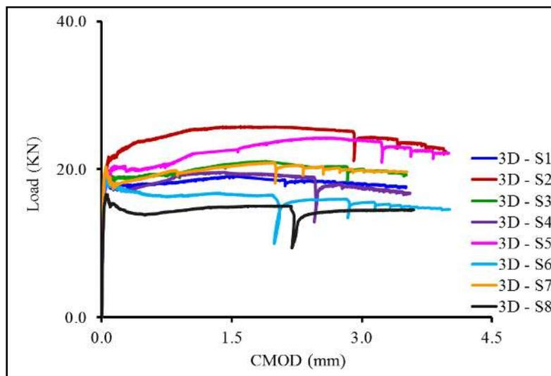
**Figure 4.1.** Load versus CMOD curves for specimens with 3D fibres (complete behaviour).
