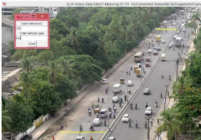
Figure 2: Screen-shot of a frame showing the study stretch in python's GUI (graphical user interface)
