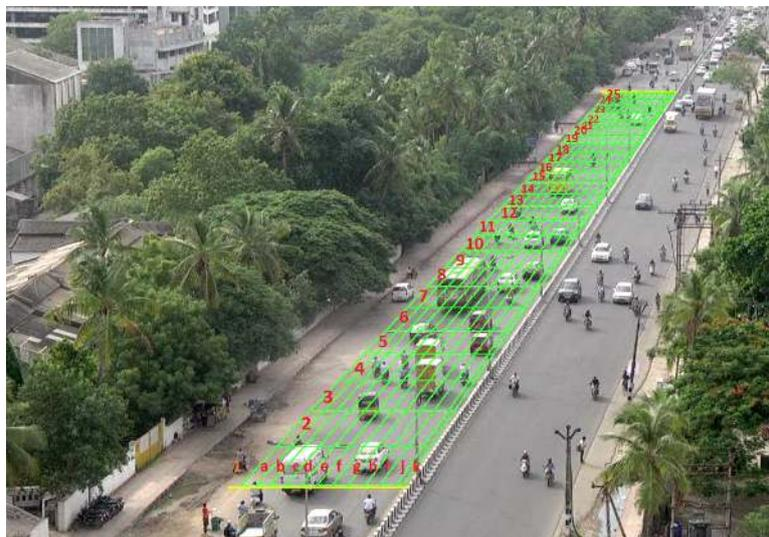
Figure 1: Grid-lines in longitudinal direction and lateral direction used for camera calibration
