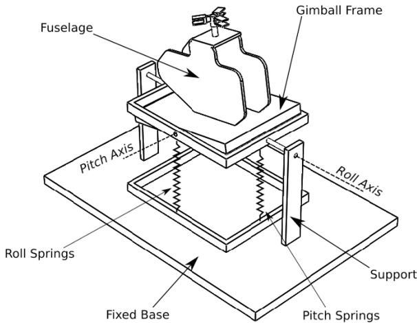
Fig. 3. Schematic of the experiment setup
