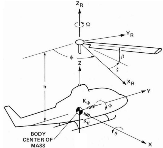
Fig. 2. Coordinate frame used in the complete analysis (Ormiston, 1991)
