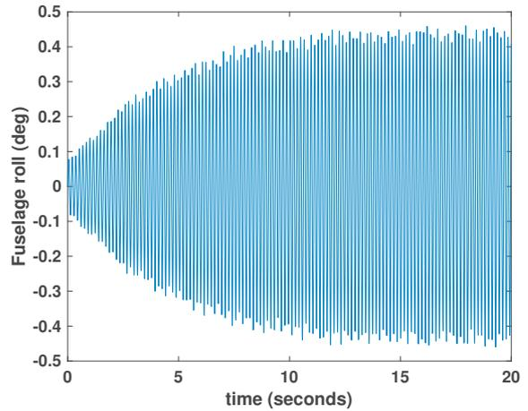
Fig. 4. Fuselage response obtained using IMU
