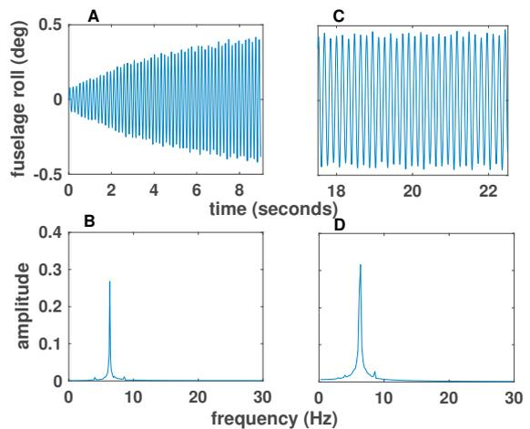
Fig. 5. Different regions of the fuselage response obtained using IMU with the corresponding frequency spectrum
