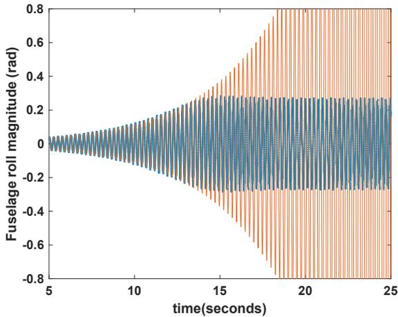
Fig. 6. Fuselage roll time response obtained using linear and nonlinear models at 760 RPM for  $\theta_0 = 0^\circ$
