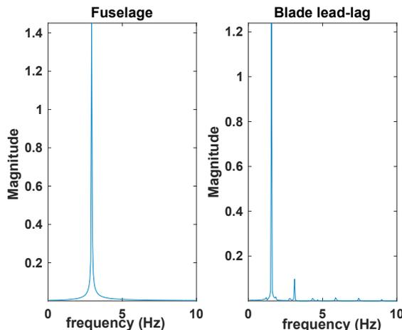
Fig. 14. Frequency spectrum of final part of fuselage and blade response (oscillations)
