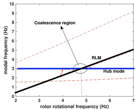
Fig. 8. Variation of modal frequency with rotor speed
