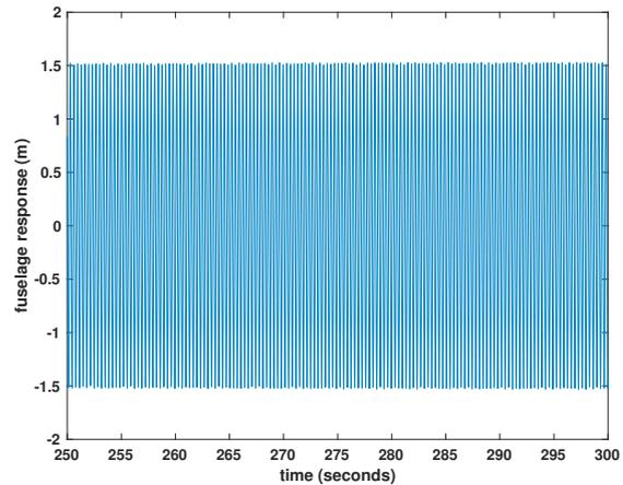
Fig. 11. Fuselage response at 4.5 Hz (final part)
