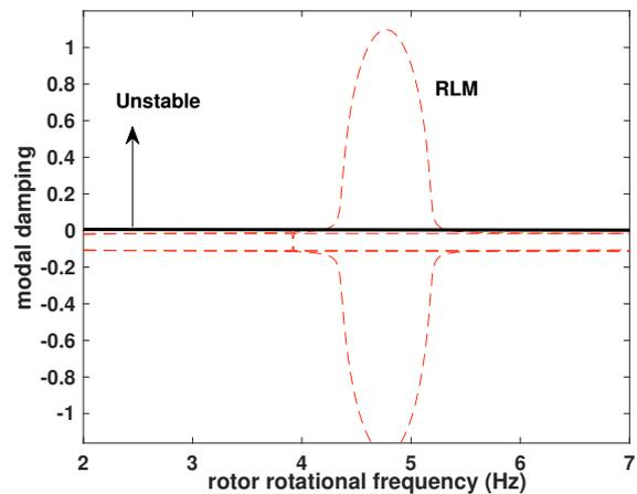
Fig. 7. Variation of modal damping with rotor speed
