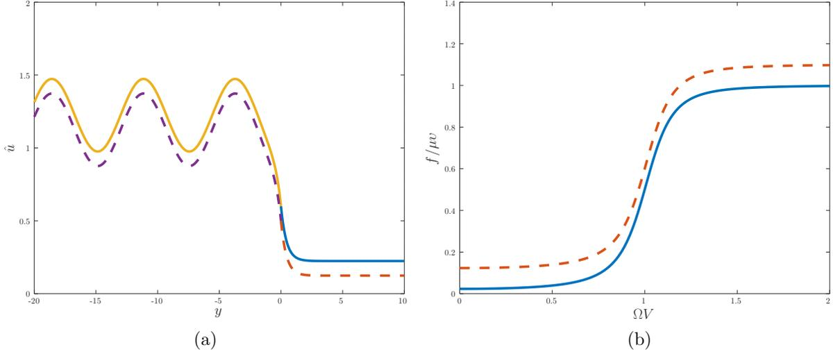
Figure 5: (a) Solution of the quasicontinuum problem for two different values of the non-dimensional temperature. Solid line is for  $\bar{\theta} = 0$  and dashed line is for  $\bar{\theta} = 0.1$ . (b) Kinetic relations for the corresponding temperatures.
