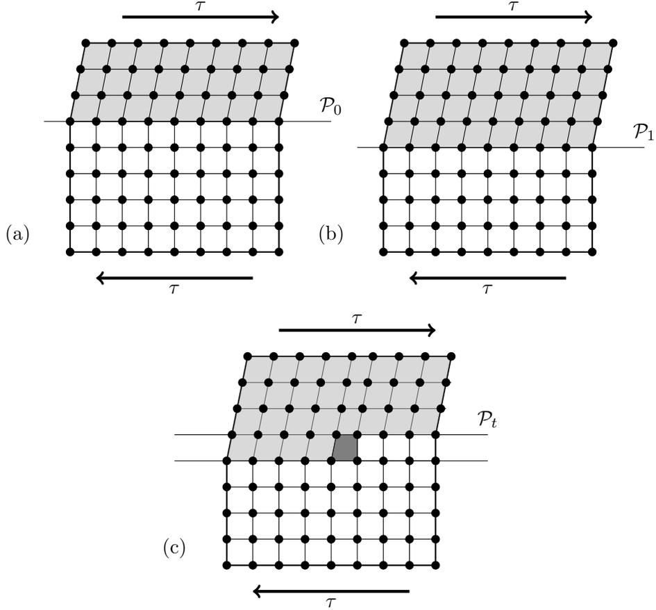
Figure 2: (a) The lattice showing the location of the phase boundary  $\mathcal{P}_0$ . (b) Phase boundary  $\mathcal{P}_1$  after motion by one lattice spacing. (c) Schematic of a ledge on the phase boundary. The ledge is shaded dark gray. The propagation of the ledge to the right results in a downward propagation of the phase boundary.
