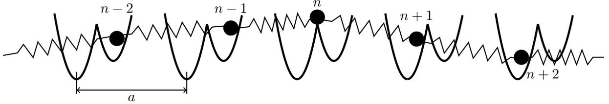
Figure 4: Frenkel-Kontorova model of the atoms on the phase boundary plane  $\mathcal{P}_t$ . Each particle experiences a substrate potential given by Eq. (11). The distance between the periodic wells is the lattice spacing of austenite  $a$ .
