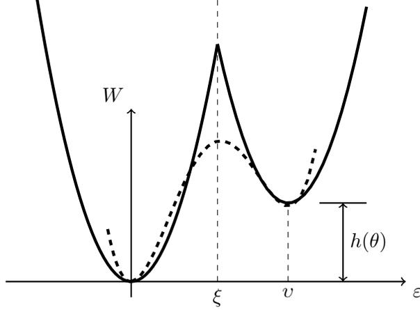
Figure 3: Energy per atom of the lattice as a function of the shear of the lattice  $\varepsilon$ . The free energy presented in Eq. (8) is shown as a function of the parameter  $\varepsilon$  as a dashed line. The solid lines represent a piecewise parabolic approximation.
