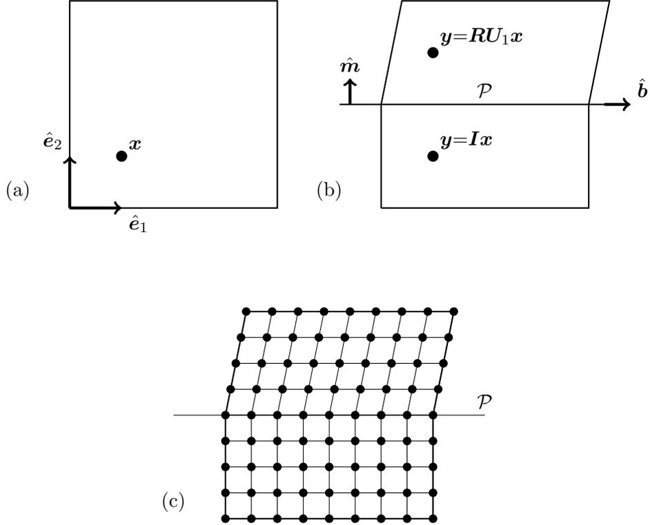
Figure 1: (a) Reference austenite configuration. (b) Partially transformed martensite. The phase boundary  $\mathcal{P}$  has a normal  $\hat{m}$ . (c) The underlying lattice in the deformed configuration.
