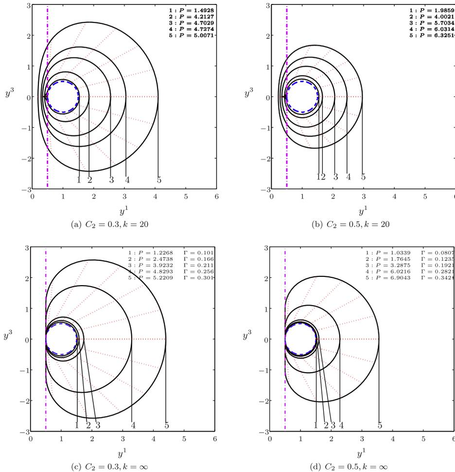
**Fig. 6.** Deformed cross-sections of a torus with  $r = 0.5$  (dashed configuration) inflating over a compliant cylinder ((a), (b)) and a rigid cylinder ((c), (d)) for certain inflation pressures. The dotted lines represent the motion of the material points during inflation, and the dot-dashed line represents the boundary of the cylindrical rim in the undeformed configuration.
