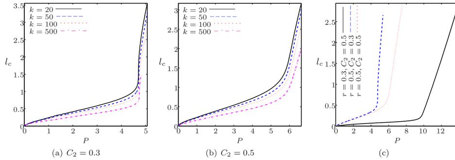
Fig. 7. Variation of the contact length with the inflation pressure for compliant ((a) and (b)) and rigid cylinder (c) cases.
