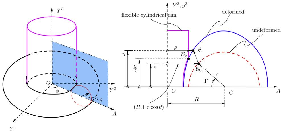
Fig. 1. A toroidal membrane in undeformed and deformed configurations over a compliant circular cylinder (modeled as a linear distributed stiffness).
