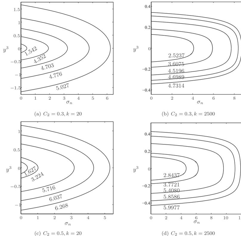
Fig. 8. The contact stress acting on the compliant cylinder in the contacting region at different inflation pressures of the toroidal membrane with material parameter values  $C_2 = 0.3, 0.5$  and stiffness values of the cylinder  $k = 20, 2500$ .
