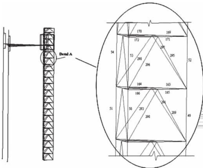
Figure 4. Finite element model for one of the legs for the jackup platform; a close up of the FE model is provided for the region around the element being studied (element number 295).
