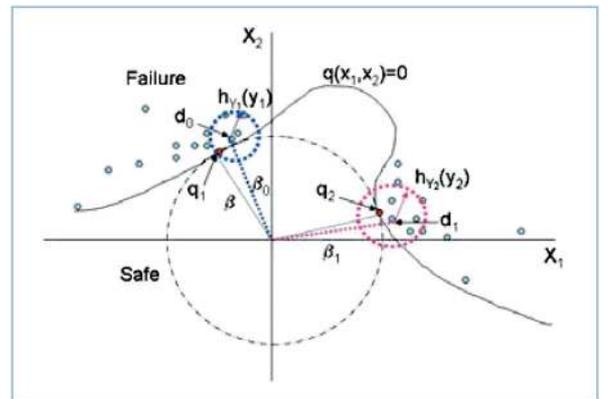
Figure 1. Schematic diagram for numerical algorithm for evaluating multidimensional integrals;  $g(x_1, x_2) = 0$  is the limit surface in the  $X_1 - X_2$  random variable space;  $h_{Y_1}(y_1)$  and  $h_{Y_2}(y_2)$  are the two importance sampling pdfs; two design points at distance  $\beta$  from the origin.
