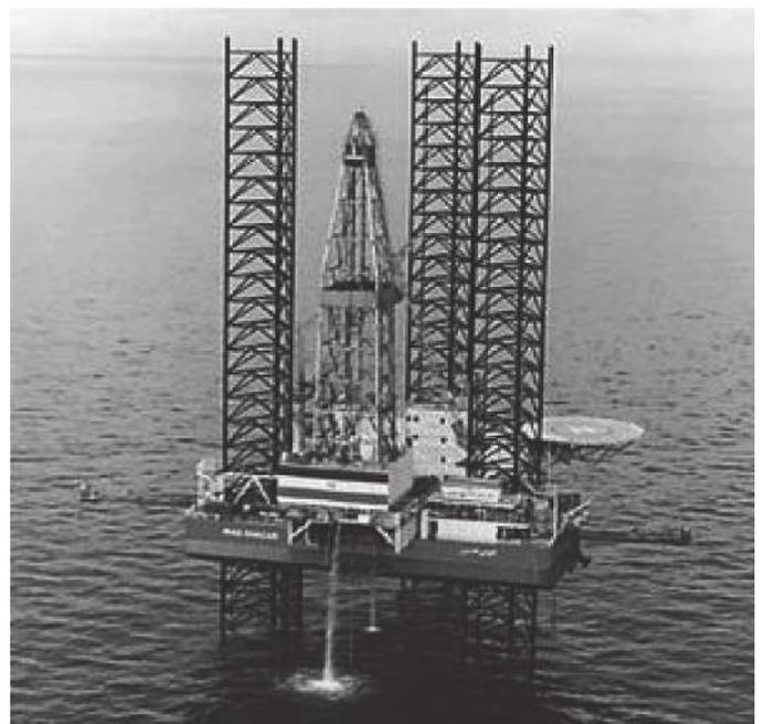
Figure 2. Jack-up platform considered in numerical example.
