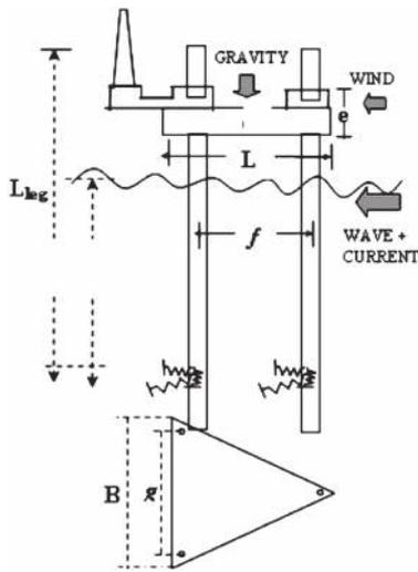
Figure 3. Schematic diagram for the elevation and the plan views for the jack-up platform.
