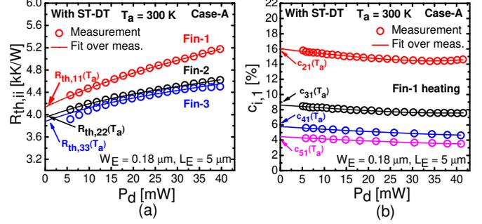
Fig. 5. Measured dissipated power-dependent (a) self-heating thermal resistance of 1<sup>st</sup>, 2<sup>nd</sup> and 3<sup>rd</sup> finger, and (b) coupling coefficients obtained when only 1<sup>st</sup> finger is heating. Extracted  $R_{th,ii}(T_a)$  and  $c_{ij}(T_a)$  are also marked.
