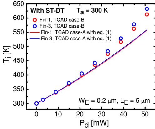
Fig. 2. Dissipated power-dependent true temperature ( $T_i$ ) of 1<sup>st</sup> and 3<sup>rd</sup> finger in a five finger transistor. Circles correspond to case-B TCAD simulation. Solid lines are the results obtained following (1) from case-A TCAD simulations by exciting one finger at a time.
