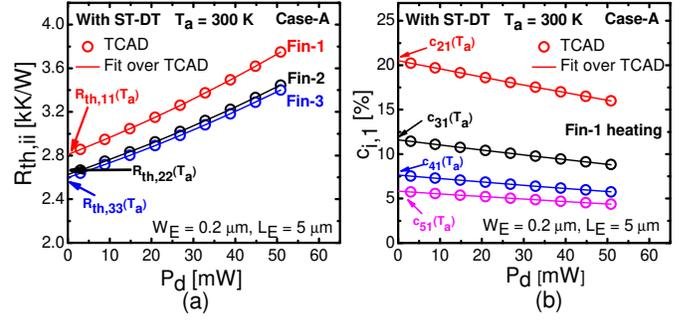
Fig. 3. Self-heating and thermal coupling results obtained from case-A TCAD simulations: (a)  $P_{d,i}$ -dependent self-heating thermal resistance  $R_{th,ii}$  of all three individually heating fingers (Fin-1, 2 and 3) and (b) coupling coefficients obtained for case-A when only 1<sup>st</sup> finger is heating ( $j = 1$ ) and rest are sensing. Ambient variables  $R_{th,ii}(T_a)$  and  $c_{ij}(T_a)$  are also indicated.
