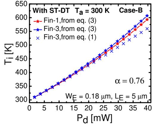
Fig. 6. Extracted values of true finger temperatures (star-lines) for 1<sup>st</sup> and 3<sup>rd</sup> finger of a five finger device from B5T technology [17]. An underestimated finger-3 temperature (crosses) obtained from a direct superposition of measured self-heating and thermal coupling temperatures is also shown for comparison.
