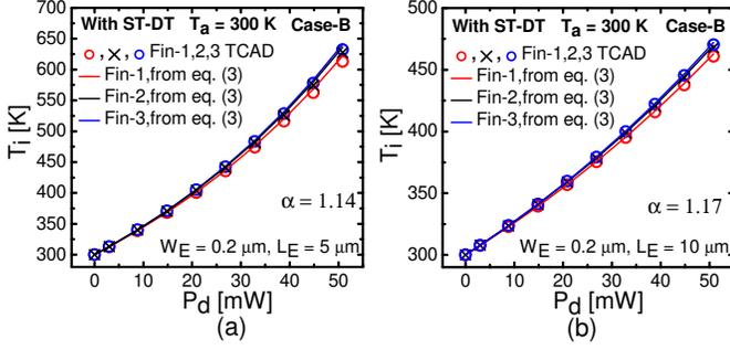
Fig. 4. A comparison of dissipated power-dependent temperatures  $T_i$ , at fingers 1, 2 and 3 obtained from the proposed extraction scheme (solid lines) against case-B TCAD simulation (symbols) for devices with emitter area ( $A_E$ ) of (a)  $A_E = 0.2 \times 5 \mu\text{m}^2$  and (b)  $A_E = 0.2 \times 10 \mu\text{m}^2$ .
