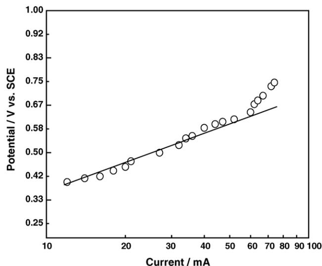
Fig. 3. Steady state polarization data obtained with a polyaniline coated stainless steel electrode (area = 0.6 cm<sup>2</sup>) in 1 M ascorbic acid + 0.5 M H<sub>2</sub>SO<sub>4</sub>.
