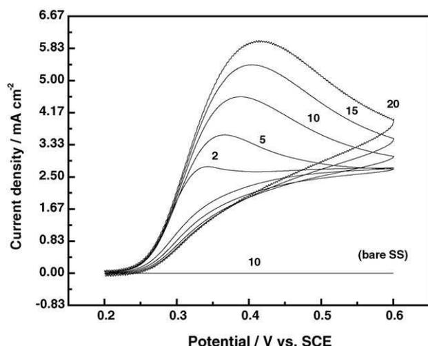
Fig. 1. Cyclic voltammograms recorded in a 50 mL solution of 10 mM Ascorbic acid + 0.5 M H<sub>2</sub>SO<sub>4</sub> with a polyaniline coated stainless steel electrode at different scan rates (mVs<sup>-1</sup>) indicated on each trace. A similar experiment was repeated for bare stainless steel electrode with a scan rate of 10 mVs<sup>-1</sup>.
