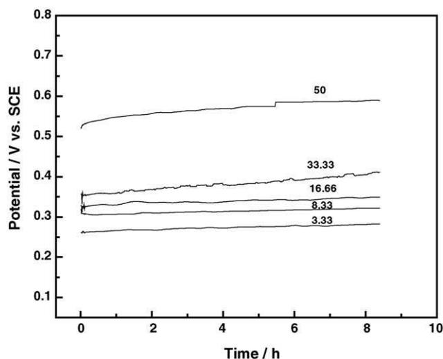
Fig. 2. Chronopotentiometry experiments performed with a polyaniline coated stainless steel electrode in 20 mL solution of 1 M ascorbic acid + 0.5 M H<sub>2</sub>SO<sub>4</sub> at different current density values (mA cm<sup>-2</sup>) indicated on each trace.
