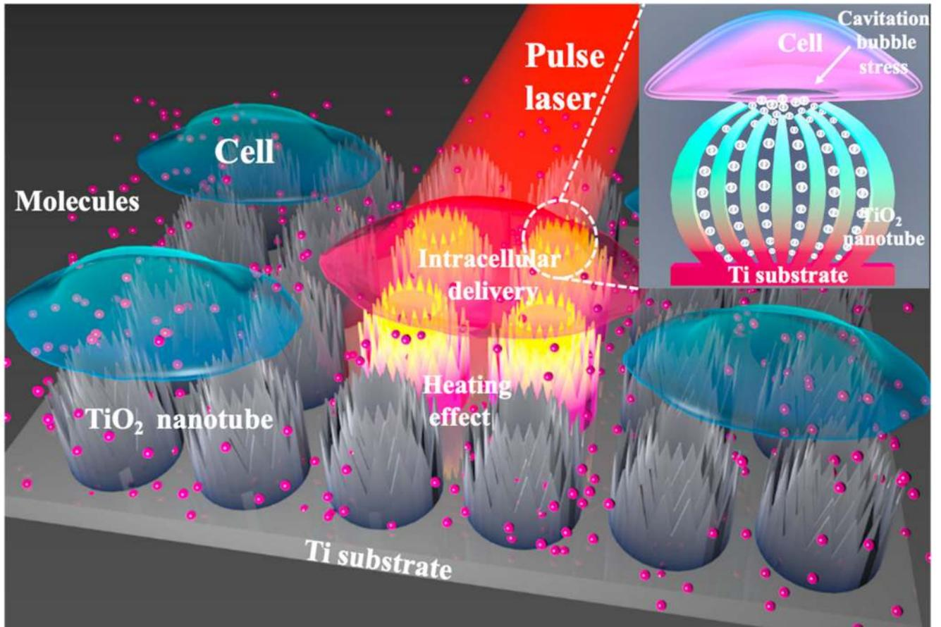
**Fig. 1.** The schematic of pulse laser-assisted vapor bubble generation and intracellular delivery using TiO<sub>2</sub> micro-flowers.
