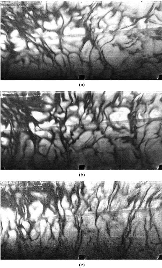
FIG. 4. Planforms of plume structure in mixed convection in air at  $Ra_w = 1.55 \times 10^8$ . (a),  $Re = 13.28 \times 10^3$ ; (b),  $Re = 14.48 \times 10^3$  and ; (c),  $Re = 15 \times 10^3$ . Flow is from top to bottom.
