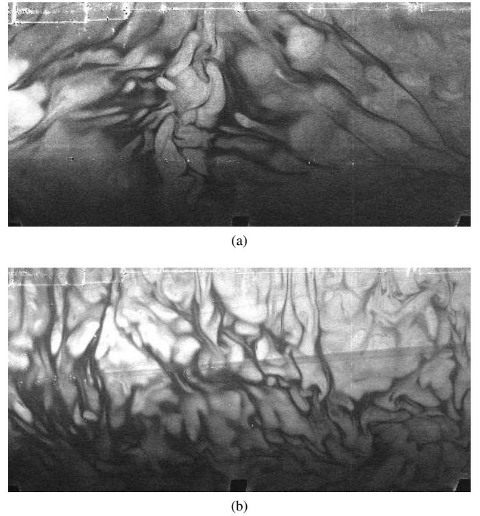
FIG. 5. Planforms of plume structure at approximately the same  $Re$  at two different  $Ra_w$  in MC in air; (a),  $Re = 9.58 \times 10^3$  at  $Ra_w = 5.75 \times 10^7$ ; (b),  $Re = 9.6 \times 10^3$  at  $Ra_w = 1.55 \times 10^8$ . Flow is from top to bottom.
