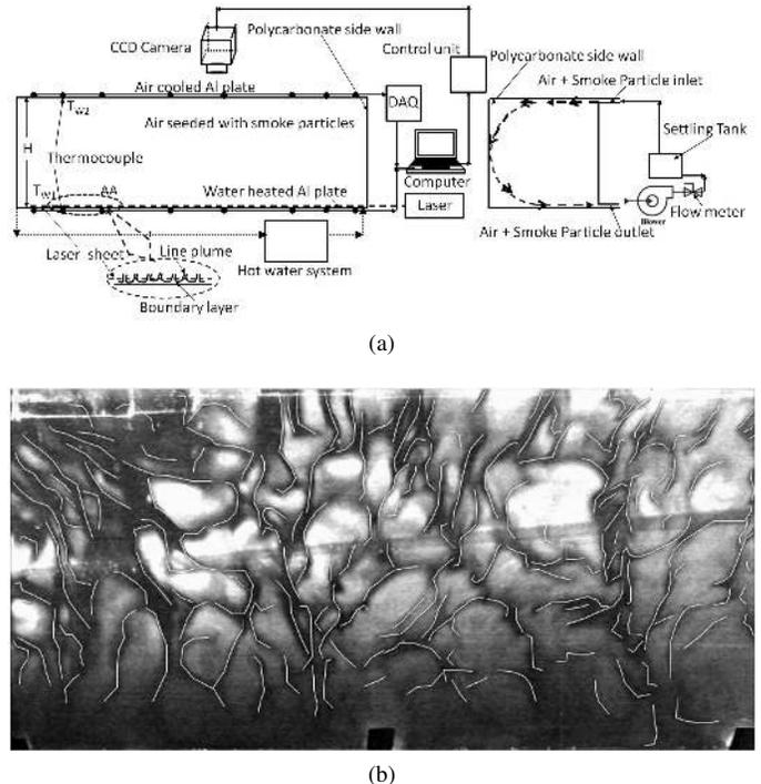
FIG. 1. (a),Schematic of the setup for steady mixed convection experiments in air at  $Pr = 0.7$ ; (b), Line plumes marked with short linear segments in the planform obtained at  $Ra_w = 1.55 \times 10^8$  and external flow rate  $Q = 1736$  lpm.
