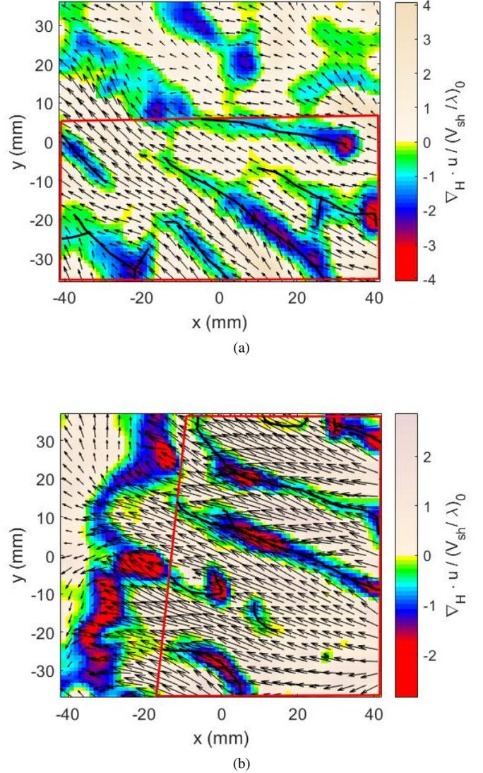
FIG. 3. Dimensionless horizontal divergence fields, overlaid over the horizontal velocity vector fields, in a horizontal plane at a height  $h_m$  from the hot surface in RBC in water. (a),  $Ra_w = 1.09 \times 10^8$ ,  $Re = 832$  and  $h_m = 1.5$  mm; (b),  $Ra_w = 6.03 \times 10^8$ ,  $Re = 2490$  and  $h_m = 1.3$  mm. Plumes are the colour regions. Shear dominant areas are shown by the red polygon.  $L_p$  is measured by adding up the length of the black lines in the plume regions.
