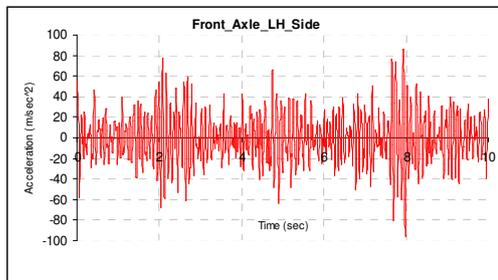
Figure 1. Pave Signal on Front Axle LH Side
