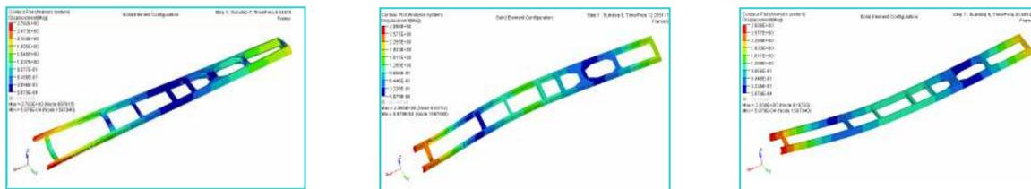
Figure 8. Fundamental Torsion, Lateral Bending and Vertical Bending Modes
