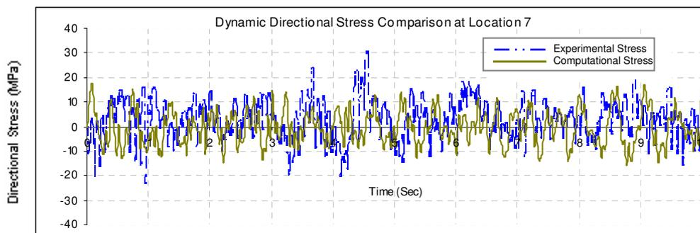
Figure 17. Experimental vs. Computational Dynamic Directional Stress at Location 7
