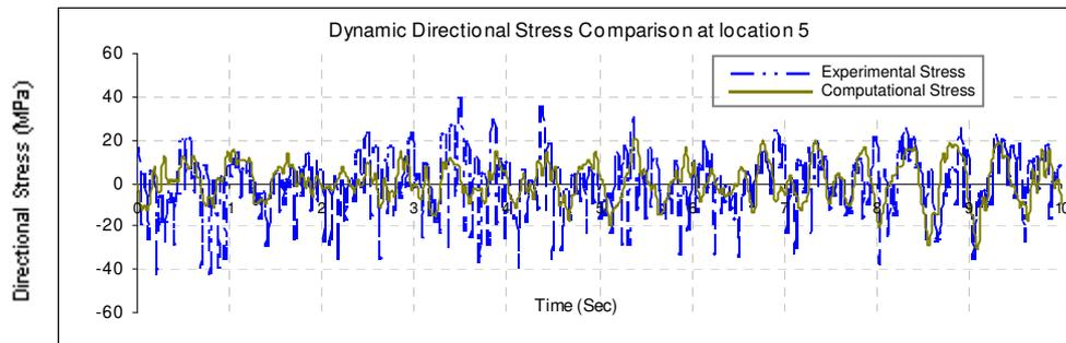
Figure 15. Experimental vs. Computational Dynamic Directional Stress at Location 5
