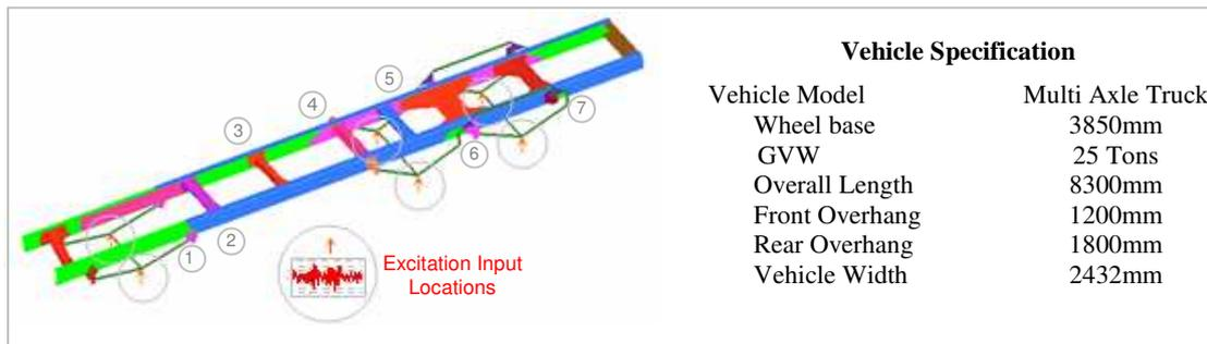
Figure 7. FE Model with Seven Strain Locations and Six Input Locations
