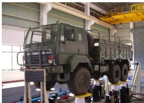
Figure 10. Six Poster Road Load Simulator
