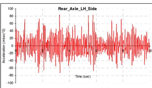
Figure 5. Pave Signal on Rear Axle LH Side
