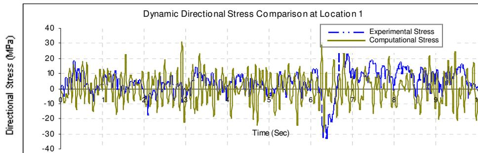
Figure 11. Experimental vs. Computational Dynamic Directional Stress at Location 1
