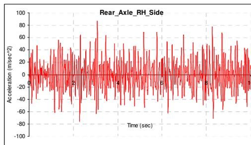
Figure 6. Pave Signal on Rear Axle RH Side
