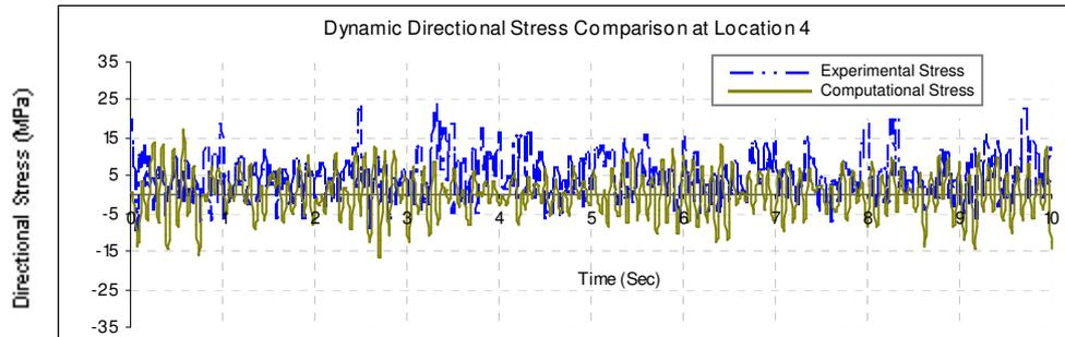
Figure 14. Experimental vs. Computational Dynamic Directional Stress at Location 4
