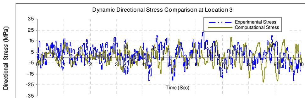
Figure 13. Experimental vs. Computational Dynamic Directional Stress at Location 3
