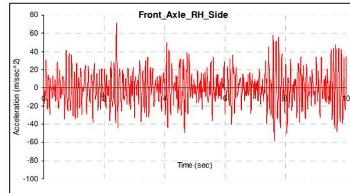
Figure 2. Pave Signal on Front Axle RH Side
