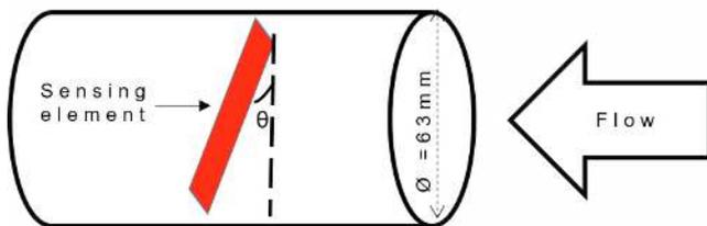
Fig. 1. Simplified schematic diagram of the proposed sensor
