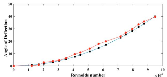
Fig. 5. Comparison between observed and cantilever model at different Reynolds number values: red- experimental; blue- theoretical
