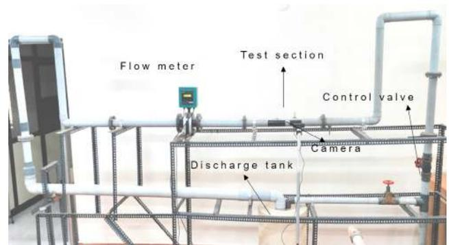
Fig. 3. Experimental system with the prototype flow sensor and a flow meter to compare the results.
