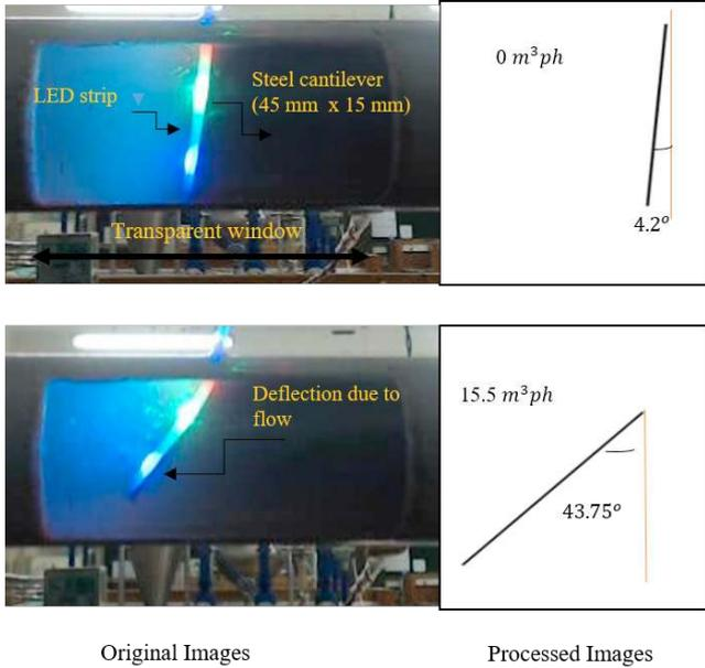
Fig. 6. Original images captured from the camera and processed images with angle from the algorithm. 4.2° offset is present in the prototype, due fixed the mechanical misalignment.
