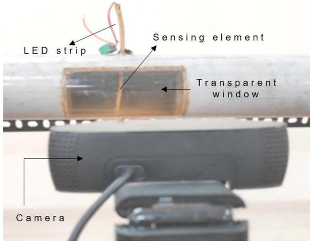
Fig. 4. Photograph of the test section
