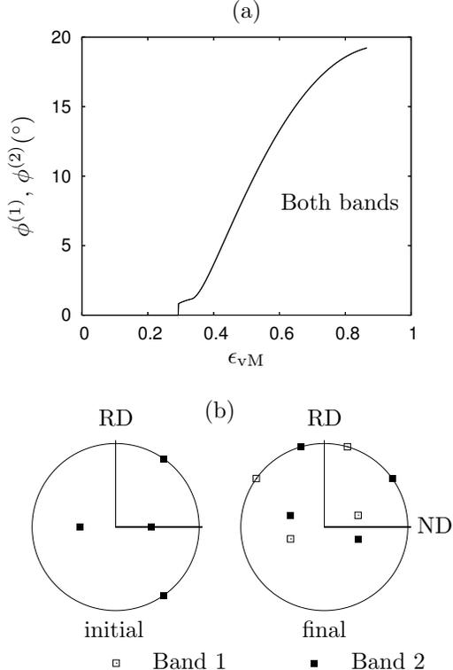
Figure 6: (a) Evolution with deformation of the middle Bunge angle in the bands ( $\phi^{(1)}$  and  $\phi^{(2)}$ ) in an initially (001)/[110]-oriented single crystal. (b) Calculated (111) pole figures before and after 75% rolling reduction. The pole figures are oriented exactly as in [34, Fig. 3] for easy comparison.
