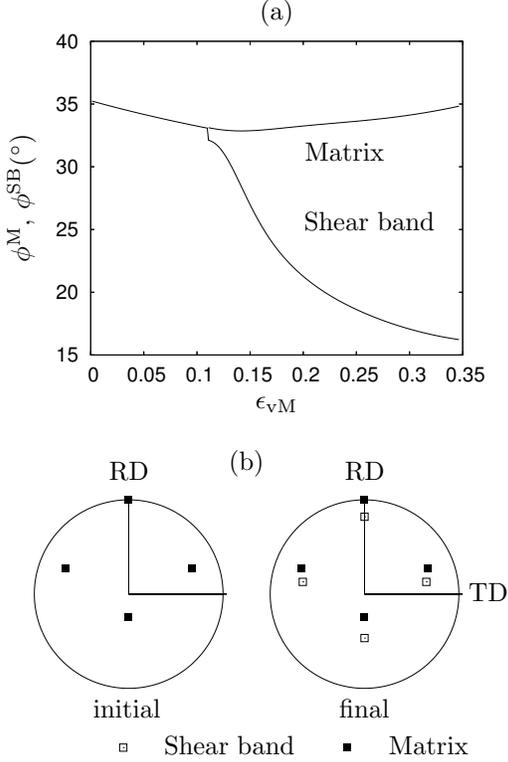
Figure 3: (a) Evolution with deformation of the middle Bunge angle in the matrix,  $(\phi^M)$  and in the shear band  $(\phi^{SB})$  in an initially C-oriented single crystal. (b) Calculated  $(111)$  pole figures before and after 30% rolling reduction. The pole figures are oriented as in [33, Fig. 3] for easy comparison.
