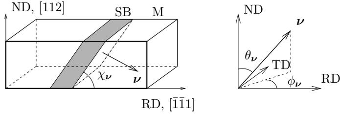
Figure 1: Initial orientation of the C-oriented crystal relative to the rolling axes. M denotes the matrix and SB the shear band. The spherical coordinates  $(\theta_\nu, \phi_\nu)$  specifying the orientation of the normal  $\nu$  to the inter-band boundary are also shown.
